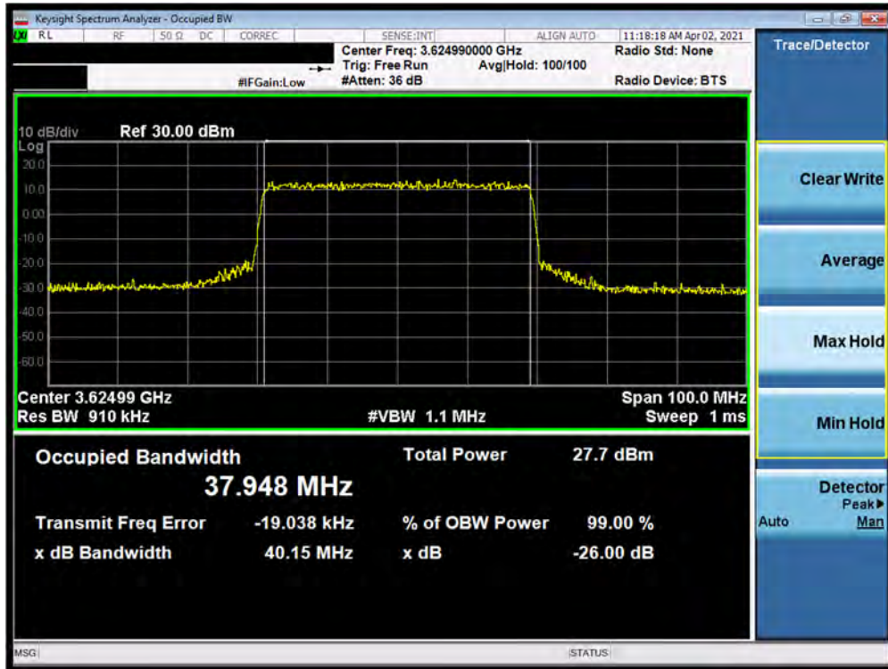
Plot 7-3. Occupied Bandwidth Plot (NR Band n48 - 40MHz 16-QAM - Full RB Configuration)
