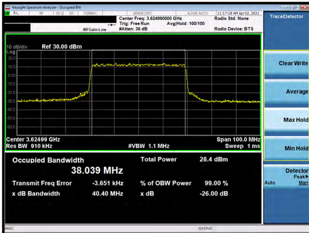
Plot 7-2. Occupied Bandwidth Plot (NR Band n48 - 40MHz QPSK - Full RB Configuration)
