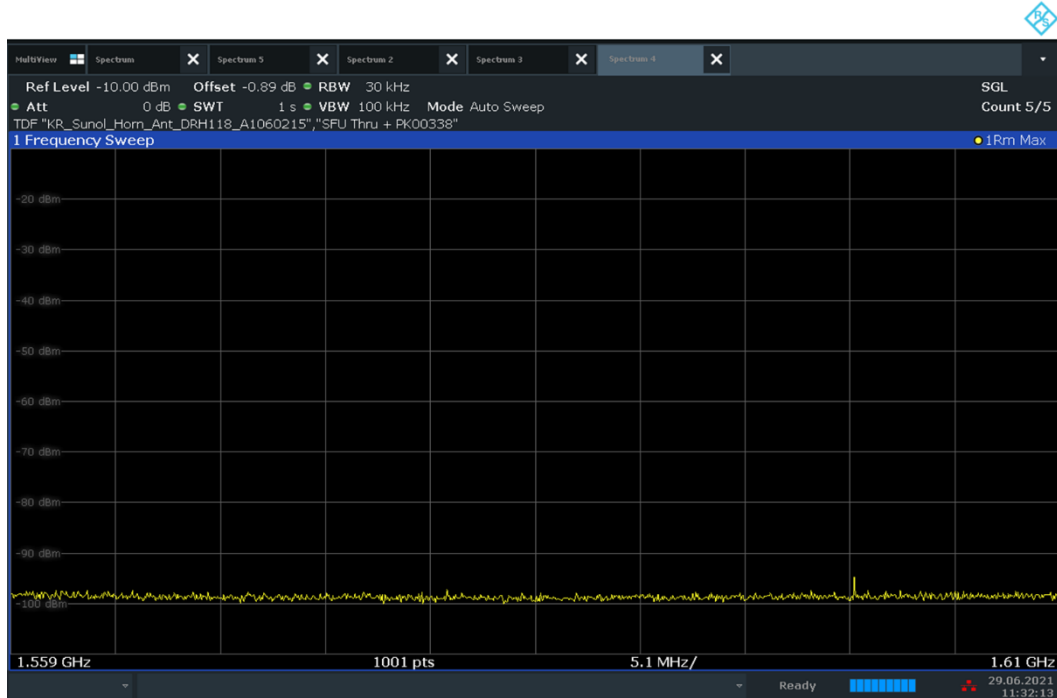
Plot 7-20. Radiated Spurious Pre-Scan 1559 - 1610 MHz - CH.5 - ANT 1 – GPS band
