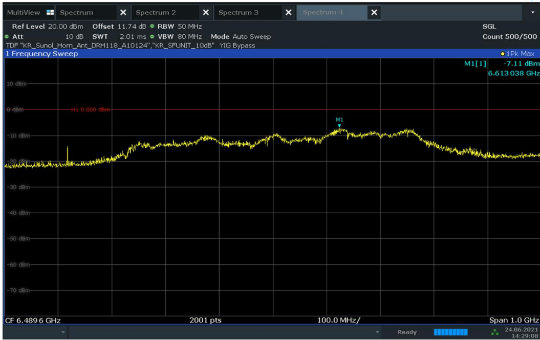
Plot 7-9. UWB Peak Power Measurement - ANT 1 - CH.5 – HPRF
