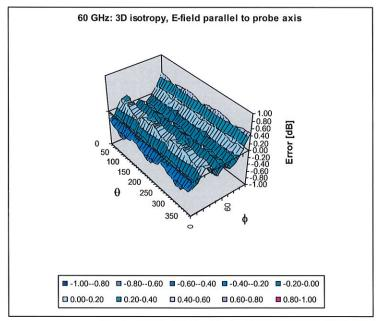
Probe isotropy for E<sub>tot</sub>: probe rotated  $\phi$  = 0° to 360°, tilted from field propagation direction  $\vec{k}$  Parallel to the field propagation ( $\psi$  =0° - 90°) at 30 GHz: deviation within ± 0.47 dB Parallel to the field propagation ( $\psi$  =0° - 90°) at 60 GHz: deviation within ± 0.49 dB
