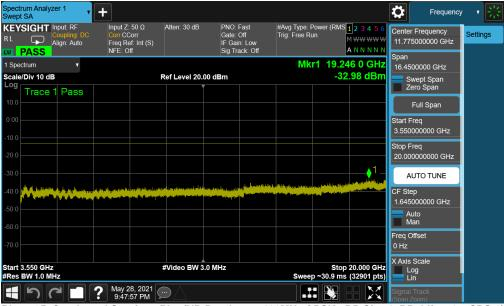
Plot 7-95. Conducted Spurious Plot (NR Band n77 - 100MHz QPSK - RB Size 1, RB Offset 0 – SRS-2)
