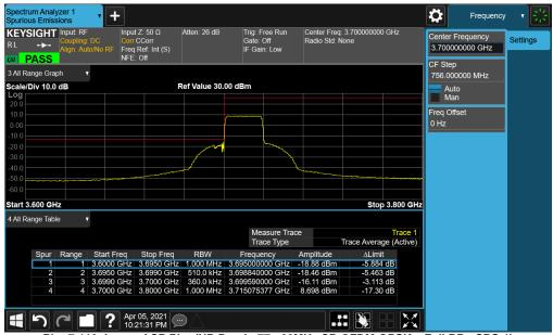
Plot 7-119. Lower ACP Plot (NR Band n77 - 20MHz CP-OFDM-QPSK - Full RB - SRS-1)
