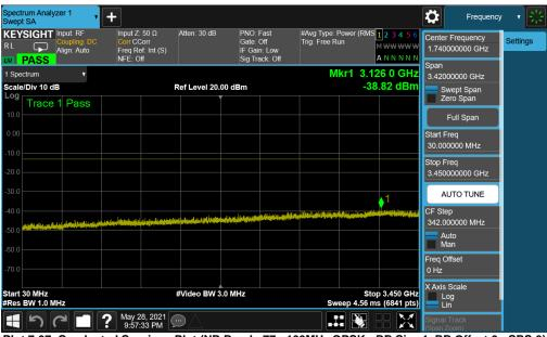
Plot 7-97. Conducted Spurious Plot (NR Band n77 - 100MHz QPSK - RB Size 1, RB Offset 0 - SRS-3)
