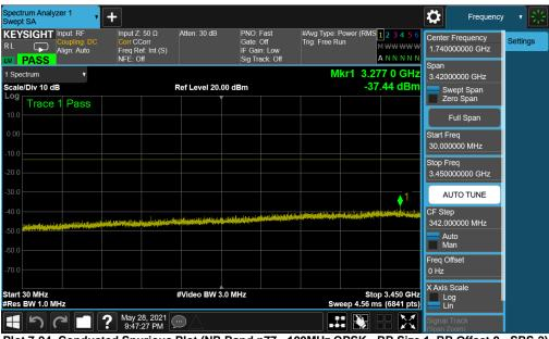
Plot 7-94. Conducted Spurious Plot (NR Band n77 - 100MHz QPSK - RB Size 1, RB Offset 0 - SRS-2)
