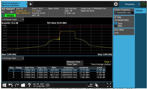
Plot 7-117. Lower ACP Plot (NR Band n77 - 30MHz CP-OFDM-QPSK - Full RB - SRS-1)
