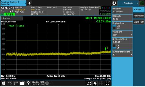
Plot 7-101. Conducted Spurious Plot (NR Band n77 - 100MHz QPSK - RB Size 1, RB Offset 0 – SRS-4)
