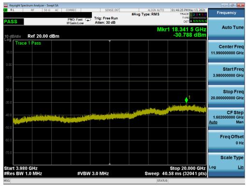
Plot 7-89. Conducted Spurious Plot (NR Band n77 - 100MHz QPSK - RB Size 1, RB Offset 0 - High Channel - SRS-4)
