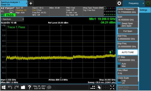
Plot 7-98. Conducted Spurious Plot (NR Band n77 - 100MHz QPSK - RB Size 1, RB Offset 0 - SRS-3)
