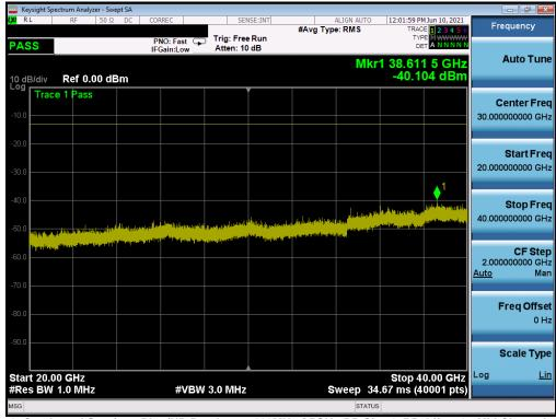
Plot 7-78. Conducted Spurious Plot (NR Band n77 - 100MHz QPSK - RB Size 1, RB Offset 0 - Mid Channel - SRS-3)
