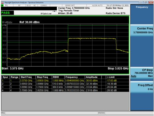
Plot 7-121. Lower ACP Plot (NR Band n77 - 100MHz CP-OFDM-QPSK - Full RB - SRS-2)
