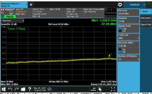
Plot 7-100. Conducted Spurious Plot (NR Band n77 - 100MHz QPSK - RB Size 1, RB Offset 0 - SRS-4)
