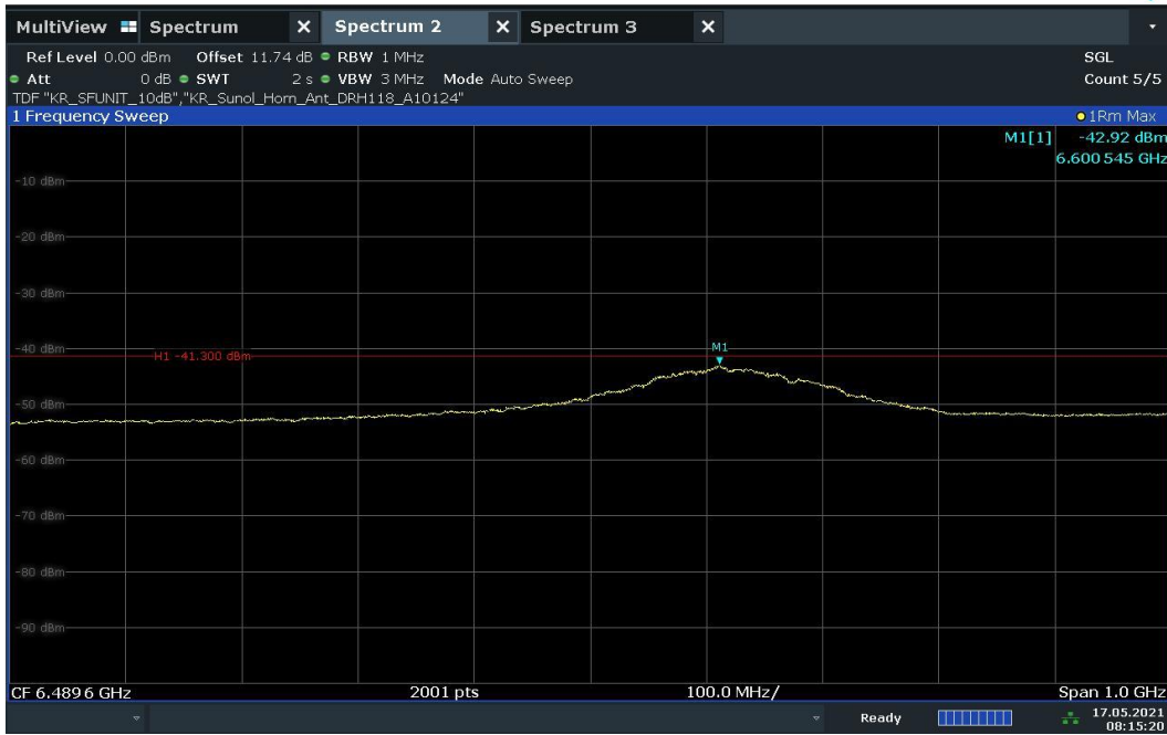
Plot 7-68. UWB Average Power Measurement - ANT 2 - CH.5 - BPRF
