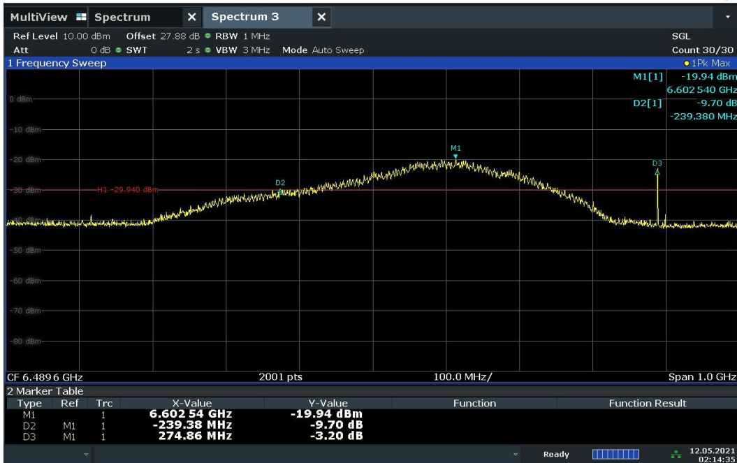
Plot 7-42. BANDWIDTH Plot – CH.5 – SP3 – Preamble 12
