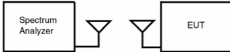
Figure 7-2. Test Instrument and Measurement Setup
