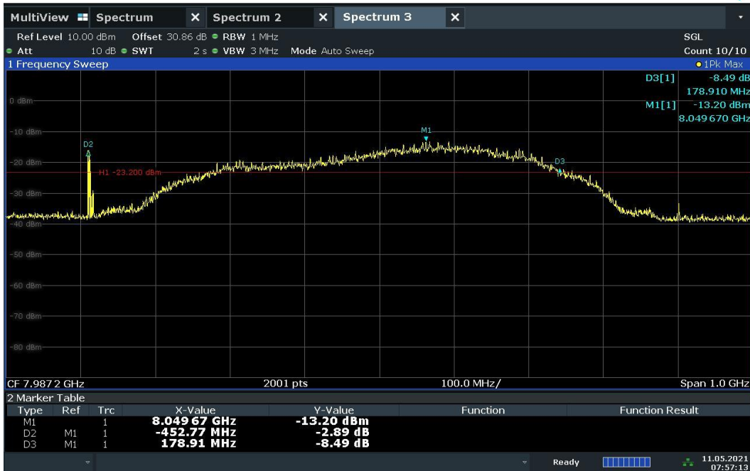
Plot 7-60. BANDWIDTH Plot – CH.9 – SP3 – Preamble 27
