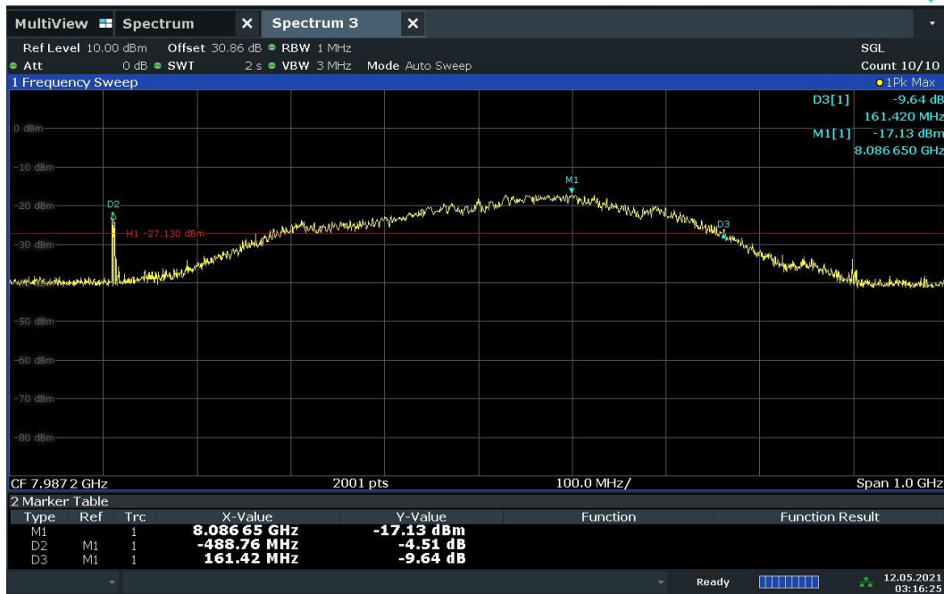
Plot 7-53. BANDWIDTH Plot – CH.9 – SP1 – Preamble 11
