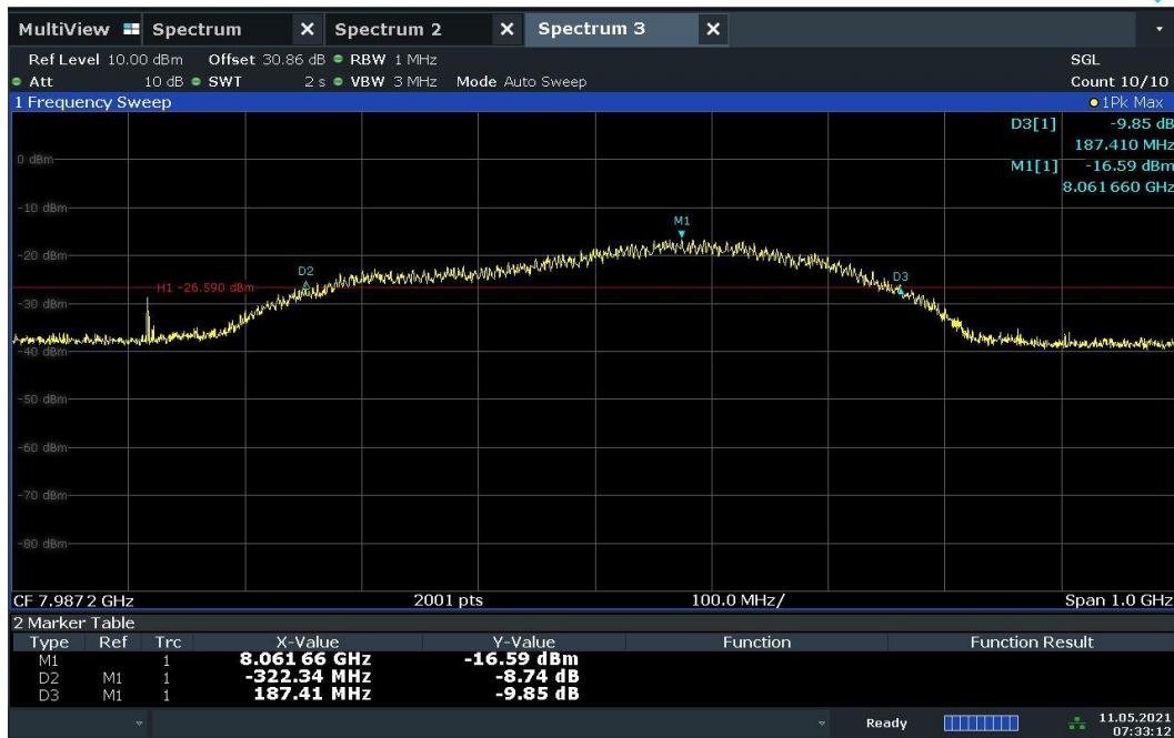
Plot 7-51. BANDWIDTH Plot – CH.9 – SP3 – Preamble 10
