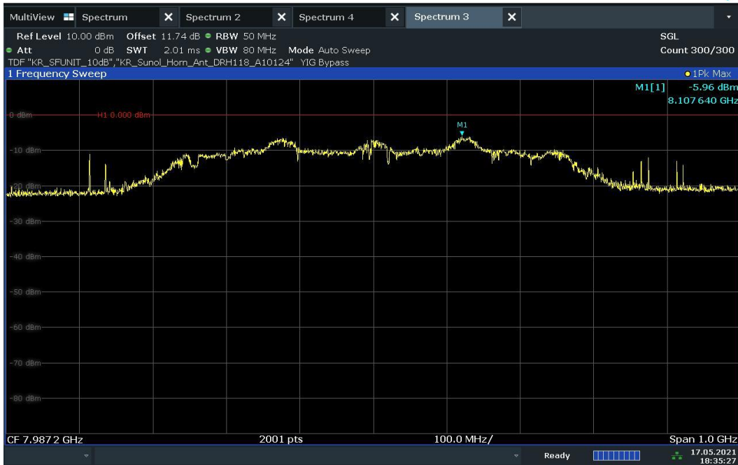
Plot 7-71. UWB Peak Power Measurement - ANT 1 - CH.9 – HPRF
