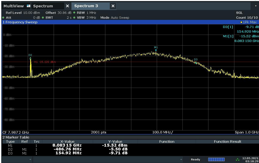
Plot 7-56. BANDWIDTH Plot – CH.9 – SP1 – Preamble 12
