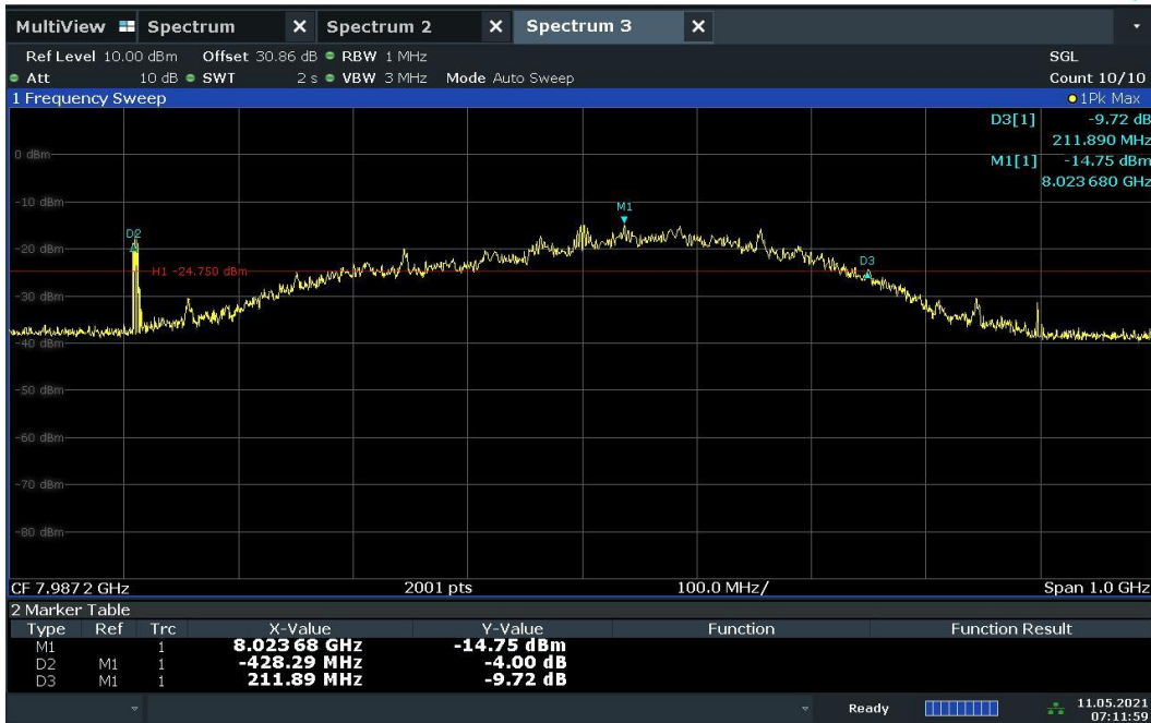
Plot 7-47. BANDWIDTH Plot – CH.9 – SP1 – Preamble 9
