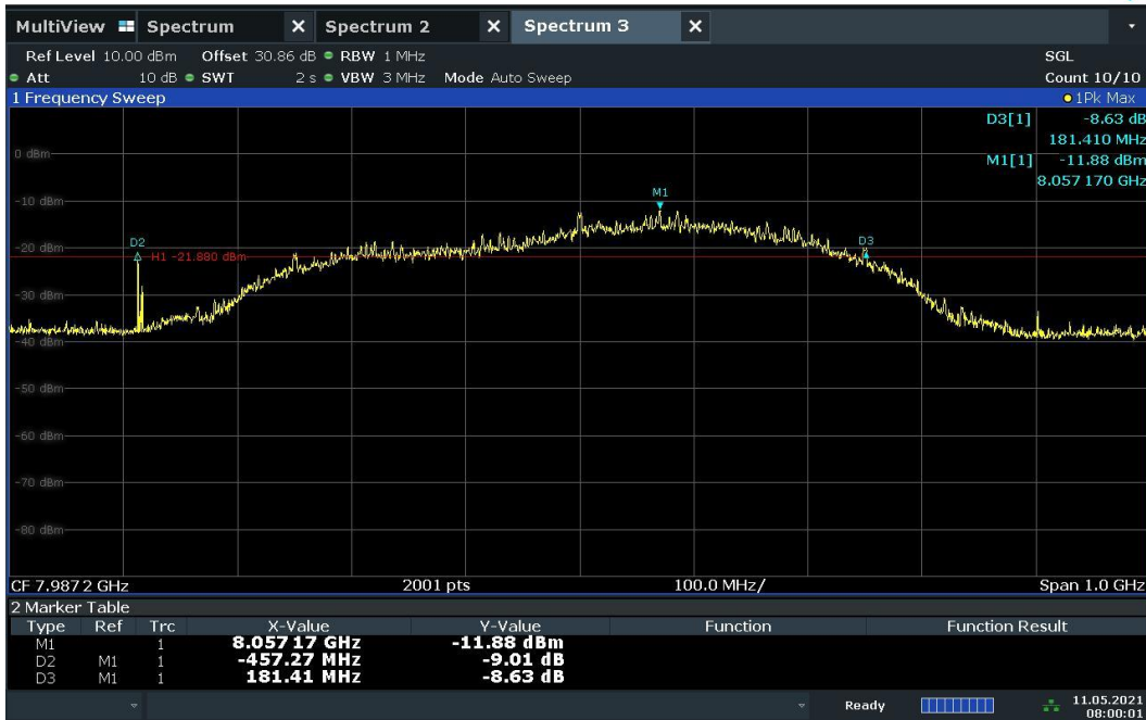
Plot 7-59. BANDWIDTH Plot – CH.9 – SP1 – Preamble 27
