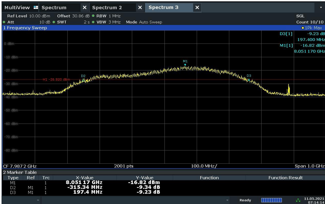
Plot 7-48. BANDWIDTH Plot – CH.9 – SP3 – Preamble 9
