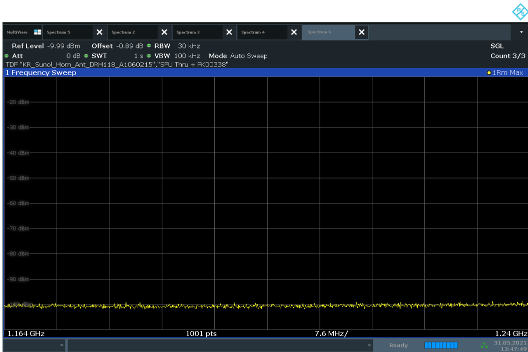
Plot 7-95. Radiated Spurious Pre-Scan 1164 - 1240 MHz - CH.9 - ANT 2 – GPS band
