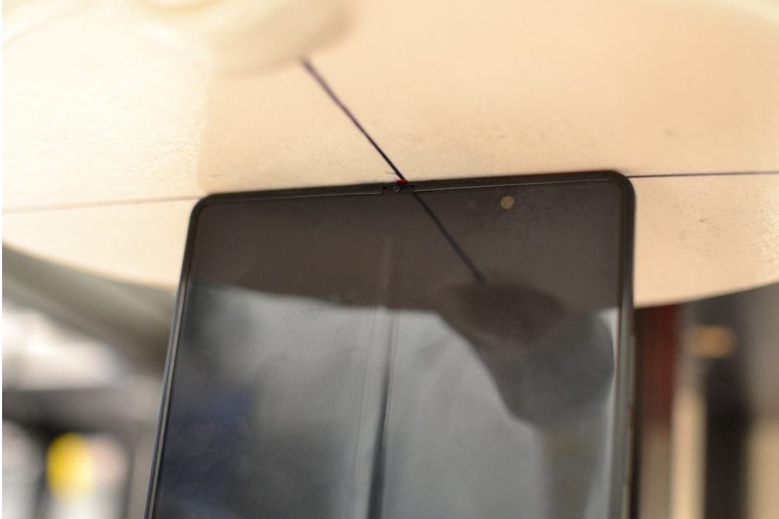
Figure C-20 SAR Test Setup Photo – UMPC Extremity, Top Edge at 0 mm
