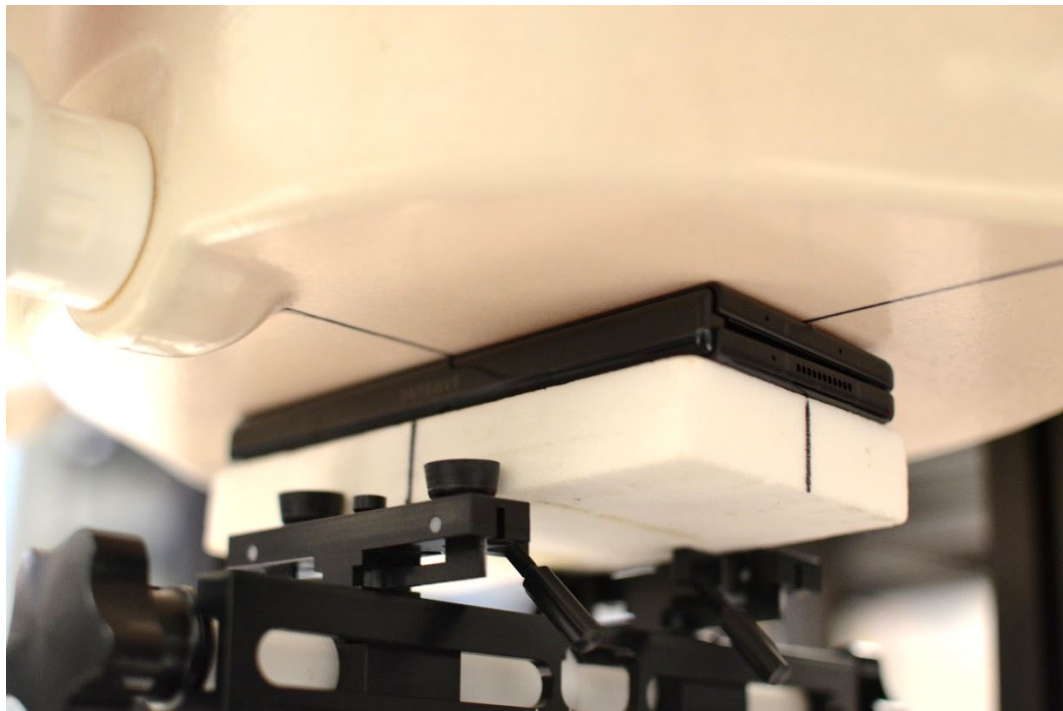
Figure C-9 SAR Test Setup Photo – Phablet, Back Side at 0 mm
