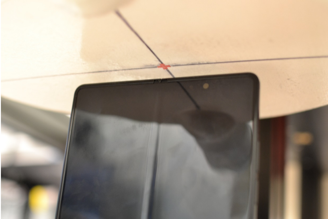
Figure C-16 SAR Test Setup Photo – UMPC Body, Top Edge at 10 mm
