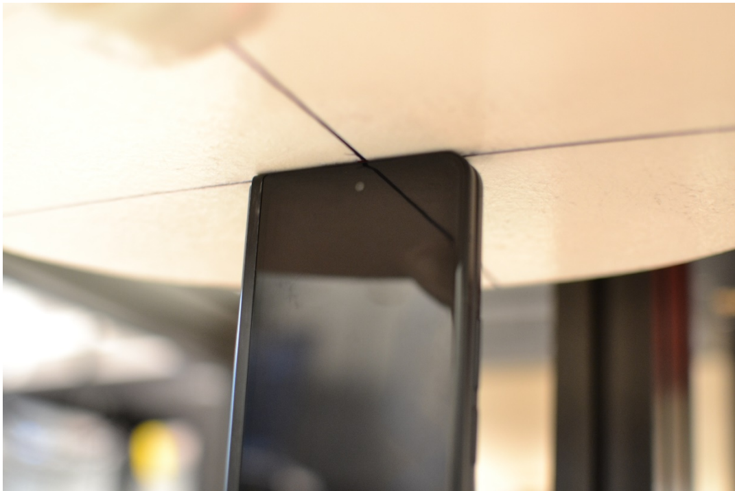
Figure C-11 SAR Test Setup Photo – Phablet, Top Edge at 0 mm
