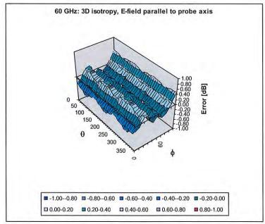
Probe isotropy for E<sub>tot</sub>: probe rotated  $\phi$  = 0° to 360°, tilted from field propagation direction  $\overline{k}$  Parallel to the field propagation ( $\psi$  =0° - 90°) at 30 GHz: deviation within ± 0.47 dB Parallel to the field propagation ( $\psi$  =0° - 90°) at 60 GHz: deviation within ± 0.49 dB
