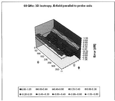
Probe isotropy for E<sub>tot</sub>: probe rotated  $\phi$  = 0° to 360°, tilted from field propagation direction  $\vec{k}$  Parallel to the field propagation ( $\psi$  =0° - 90°) at 30 GHz: deviation within ± 0.34 dB Parallel to the field propagation ( $\psi$  =0° - 90°) at 60 GHz: deviation within ± 0.35 dB
