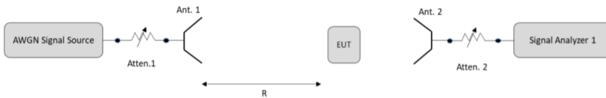
Figure 7-6. Test Instrument & Measurement Setup – Detection Threshold Measurement
