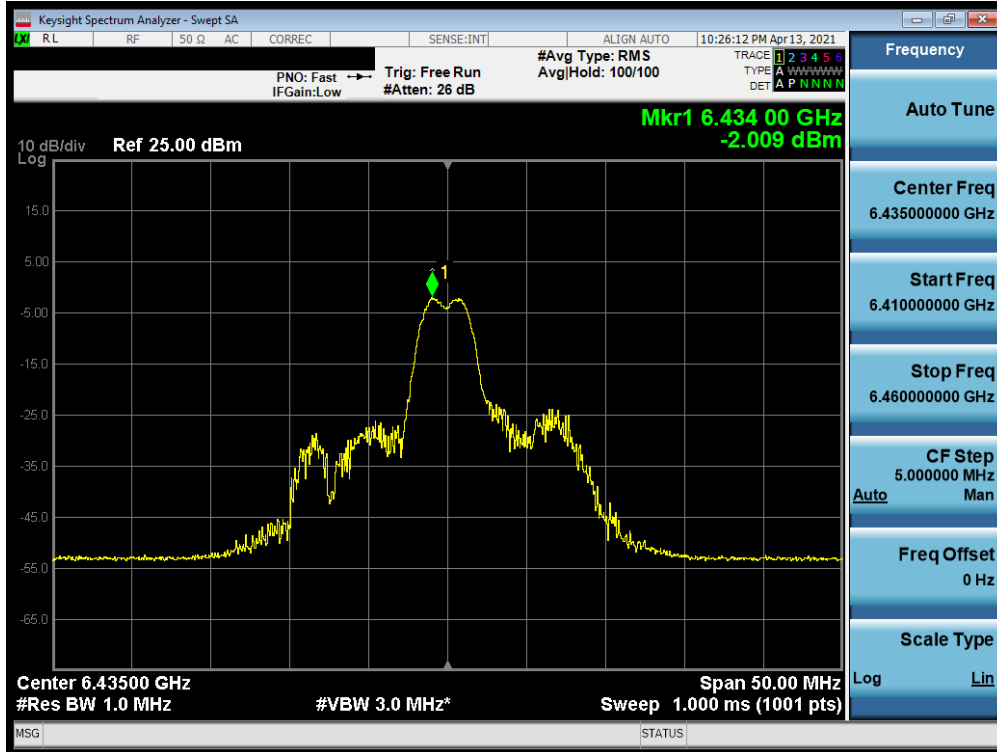
Plot 7-152. Power Spectral Density Plot MIMO ANT1 (20MHz BW 802.11ax (26 Tones) (UNII Band 6) – Ch. 97)
