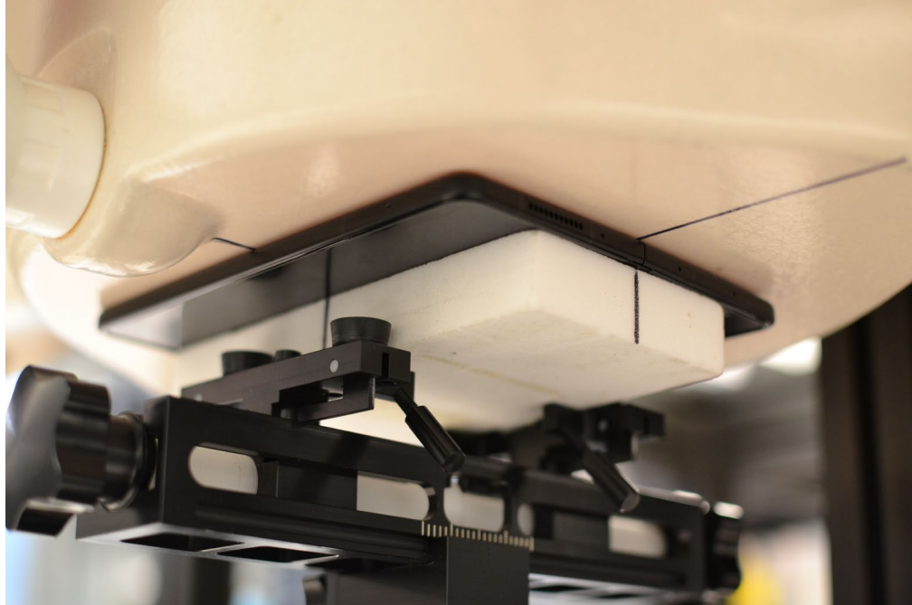
SAR Test Setup Photo 21– Open Configuration (UMPC), UMPC Extremity, Back Side, 0 mm
