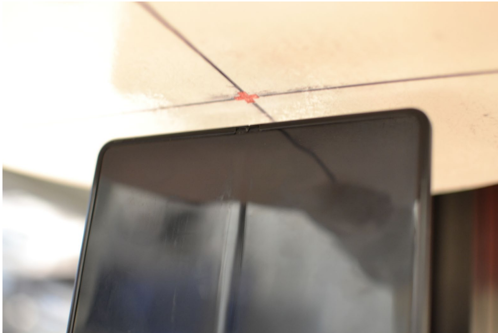
SAR Test Setup Photo 28– Open Configuration (UMPC), UMPC Body, Bottom Edge, 10 mm
