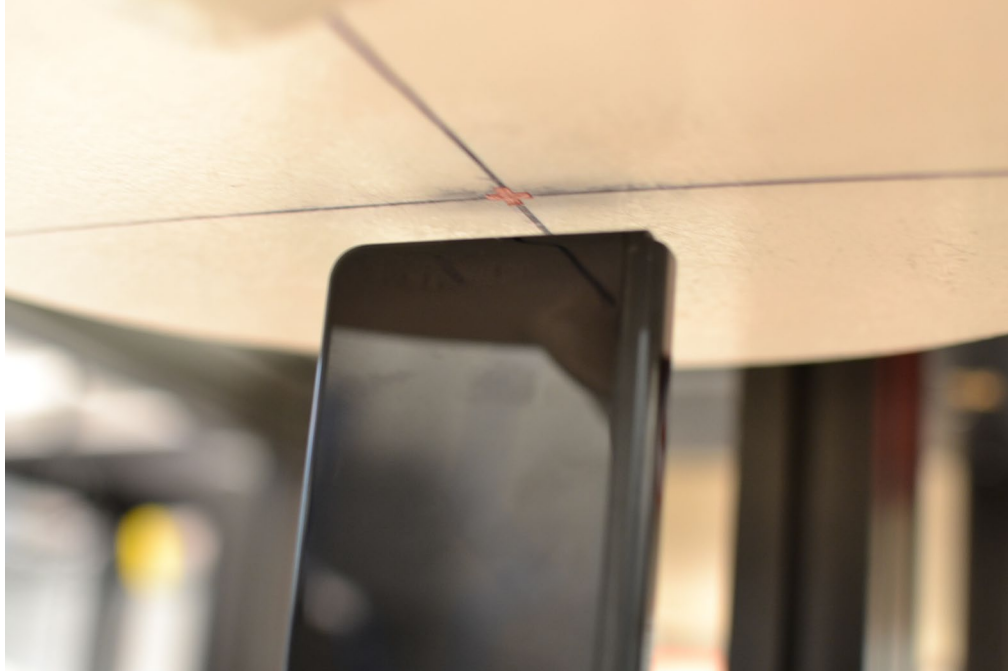
SAR Test Setup Photo 13– Closed Configuration (Handset), Hotspot, Bottom Edge, 10 mm
