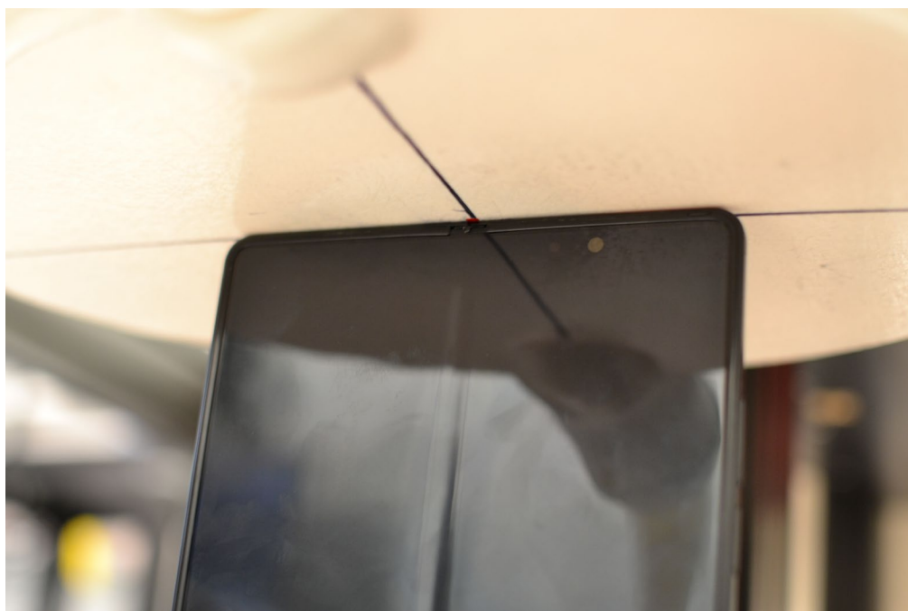
SAR Test Setup Photo 26– Open Configuration (UMPC), UMPC Extremity, Top Edge, 0 mm
