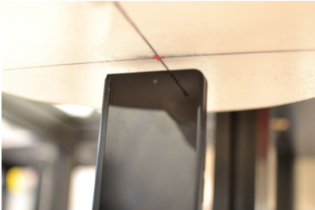
SAR Test Setup Photo 10– Closed Configuration (Handset), Hotspot, Top Edge, 10 mm
