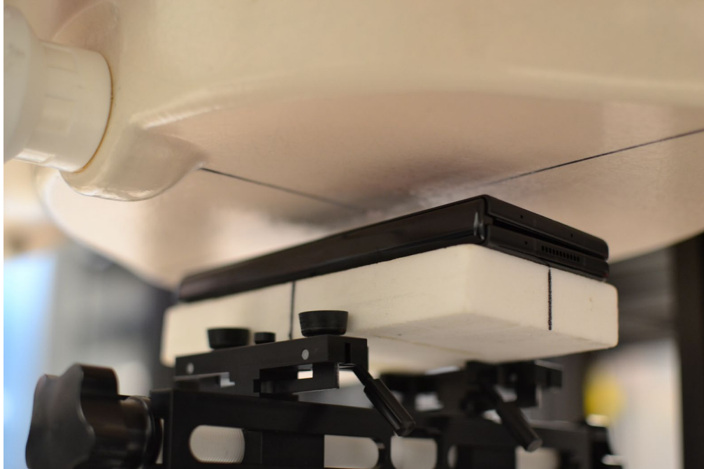
SAR Test Setup Photo 5– Closed Configuration (Handset), Body-worn, Back Side, 15 mm
