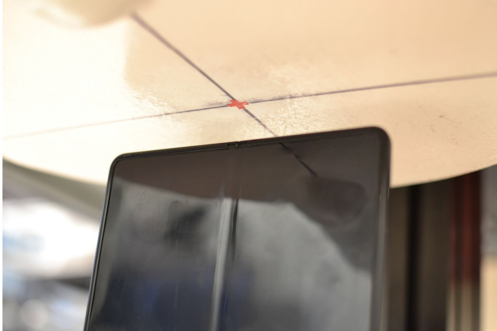
SAR Test Setup Photo 27– Open Configuration (UMPC), UMPC Body/Extremity, Bottom Edge, 16 mm
