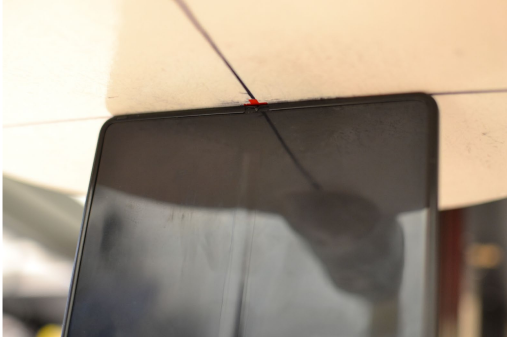
SAR Test Setup Photo 29– Open Configuration (UMPC), UMPC Extremity, Bottom Edge, 0 mm
