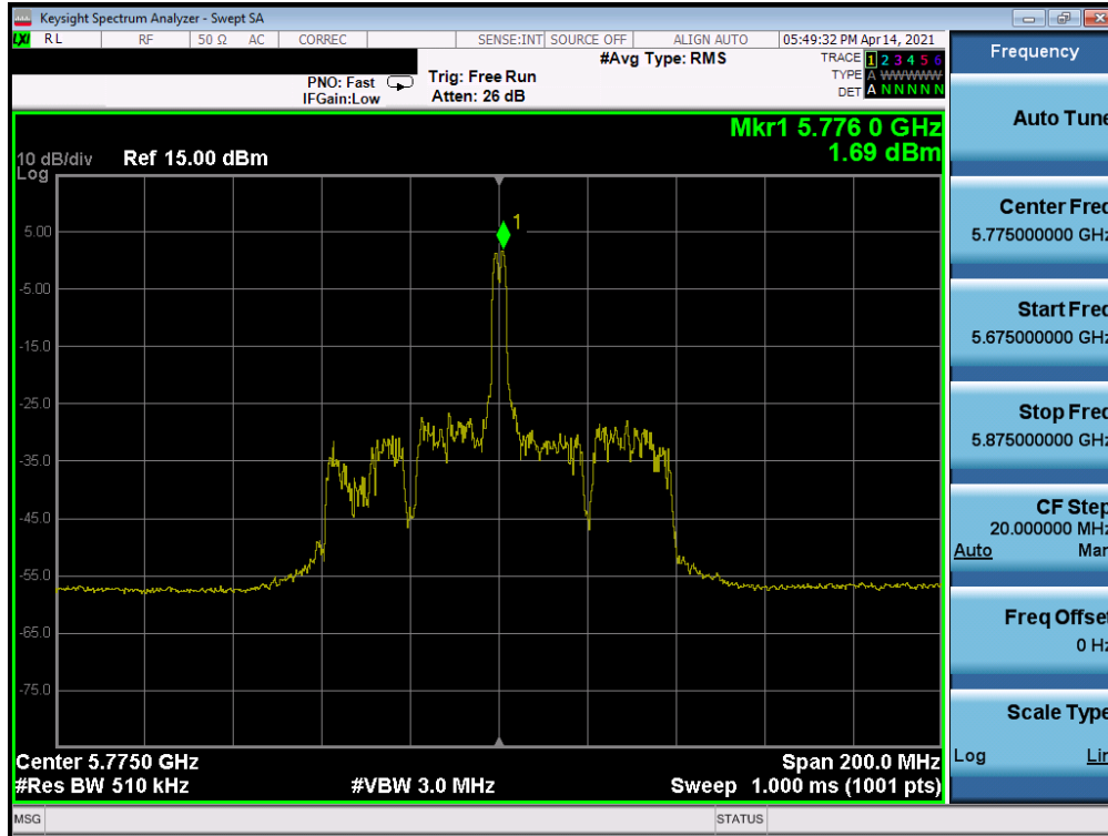
Plot 7-217. Power Spectral Density Plot MIMO ANT2 (80MHz BW 802.11ax – 26 Tones (UNII Band 3) – Ch. 155)
