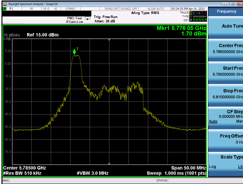
Plot 7-213. Power Spectral Density Plot MIMO ANT2 (20MHz BW 802.11ax – 26 Tones (UNII Band 3) – Ch. 157)
