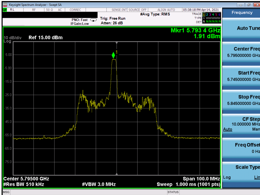
Plot 7-216. Power Spectral Density Plot MIMO ANT2 (40MHz BW 802.11ax – 26 Tones (UNII Band 3) – Ch. 159)
