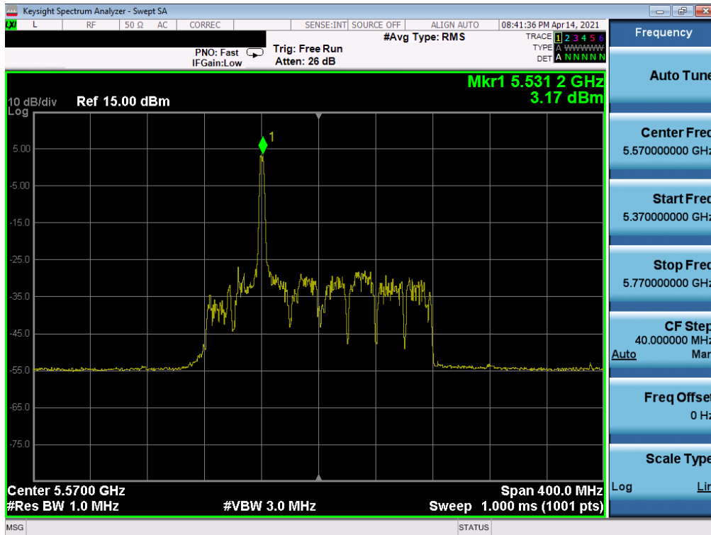
Plot 7-210. Power Spectral Density Plot MIMO ANT2 (160MHz BW(L) 802.11ax – 26 Tones (UNII Band 2C) – Ch. 114)
