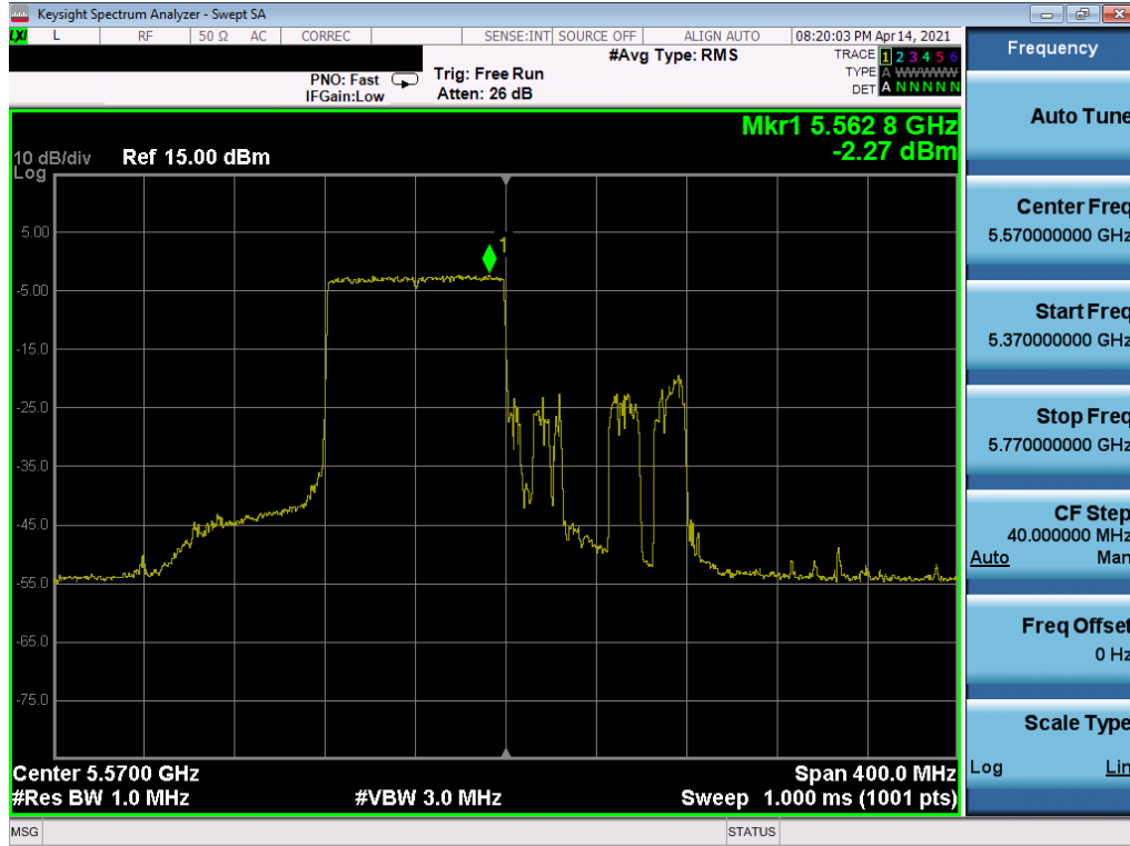
Plot 7-179. Power Spectral Density Plot MIMO ANT1 (160MHz BW(L) 802.11ax – Full Tones (UNII Band 2C) – Ch. 114)
