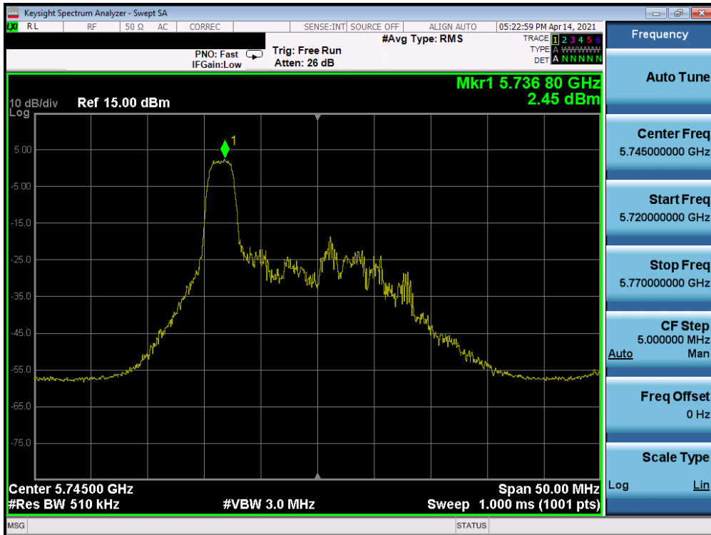
Plot 7-212. Power Spectral Density Plot MIMO ANT2 (20MHz BW 802.11ax – 26 Tones (UNII Band 3) – Ch. 149)
