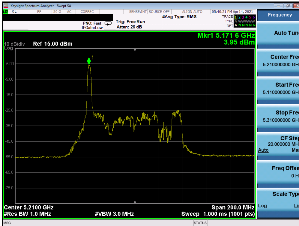
Plot 7-192. Power Spectral Density Plot MIMO ANT2 (80MHz BW 802.11ax – 26 Tones (UNII Band 1) – Ch. 42)
