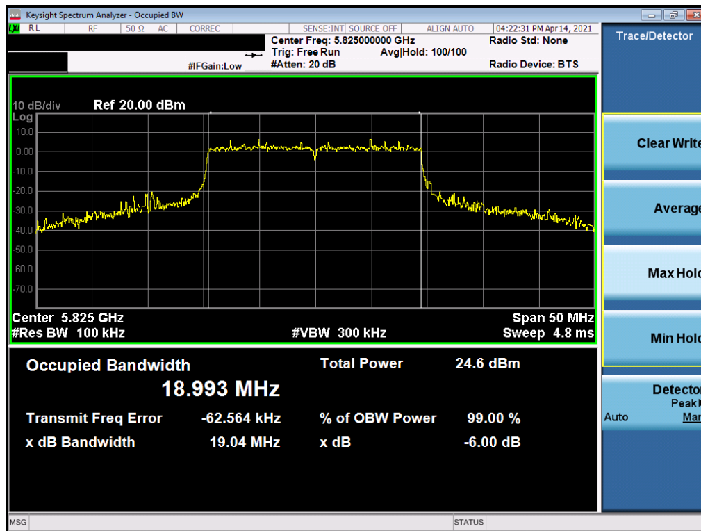
Plot 7-115. 6dB Bandwidth Plot MIMO ANT1 (20MHz BW 802.11ax – 242 Tones (UNII Band 3) – Ch. 165)
