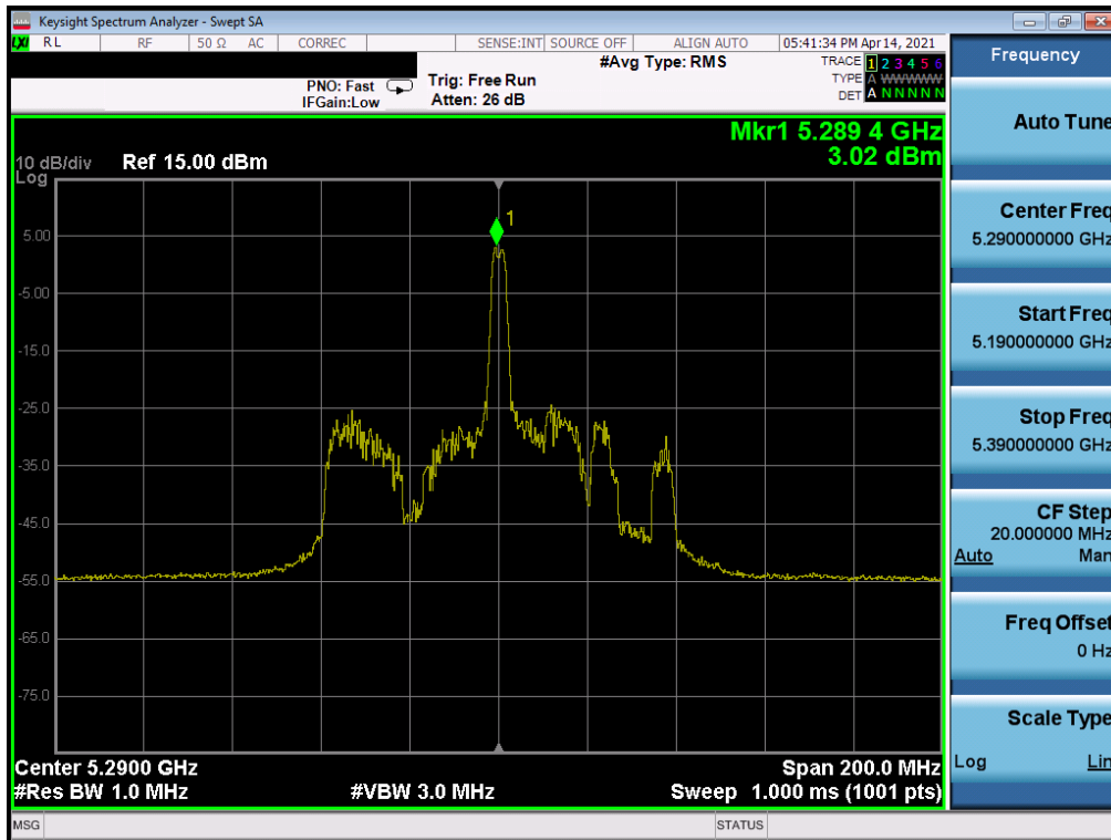
Plot 7-200. Power Spectral Density Plot MIMO ANT2 (80MHz BW 802.11ax – 26 Tones (UNII Band 2A) – Ch. 58)
