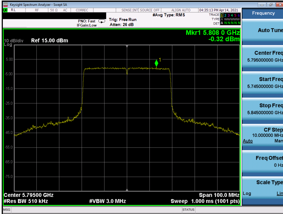
Plot 7-185. Power Spectral Density Plot MIMO ANT1 (40MHz BW 802.11ax – Full Tones (UNII Band 3) – Ch. 159)
