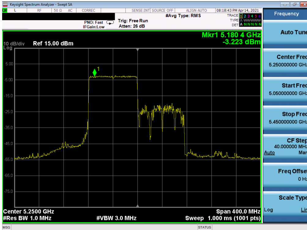
Plot 7-162. Power Spectral Density Plot MIMO ANT1 (160MHz BW(L) 802.11ax – Full Tones (UNII Band 1/2A) – Ch. 50)
