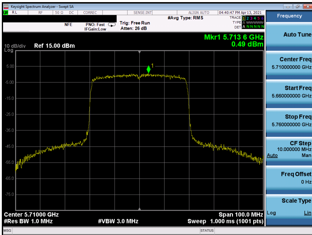
Plot 7-327. Power Spectral Density Plot MIMO ANT1 (40MHz BW 802.11ax (UNII Band 2C) – Ch. 142)
