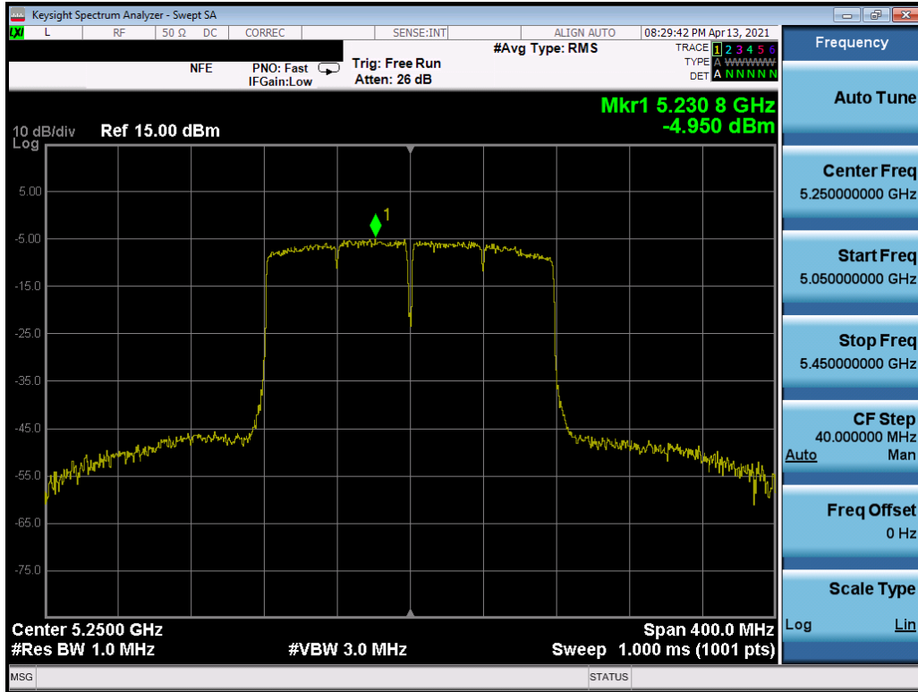
Plot 7-296. Power Spectral Density Plot MIMO ANT1 (160MHz BW 802.11ac (UNII Band 1/2A) – Ch. 50)
