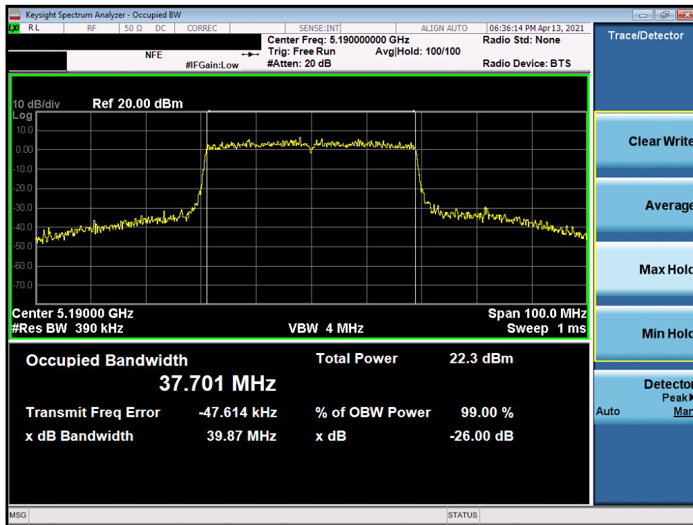
Plot 7-122. 26dB Bandwidth Plot MIMO ANT2 (40MHz BW 802.11ax (UNII Band 1) – Ch. 38)
