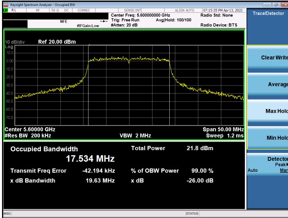
Plot 7-147. 26dB Bandwidth Plot MIMO ANT2 (20MHz BW 802.11n (UNII Band 2C) – Ch. 120)
