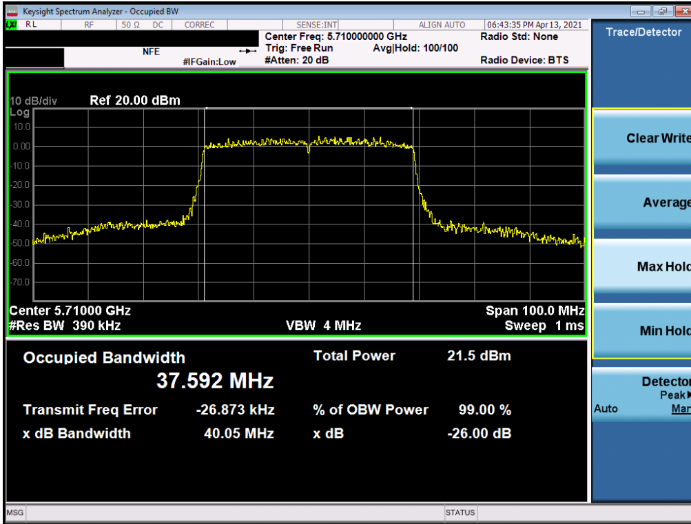
Plot 7-157. 26dB Bandwidth Plot MIMO ANT2 (40MHz BW 802.11ax (UNII Band 2C) – Ch. 142)
