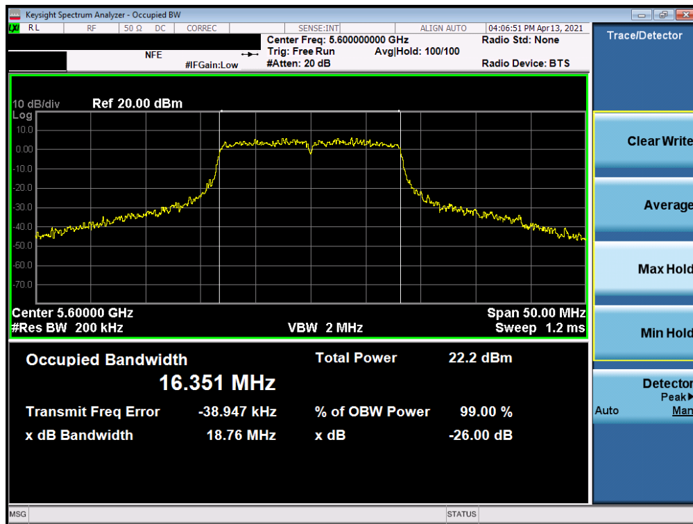
Plot 7-89. 26dB Bandwidth Plot MIMO ANT1 (802.11a (UNII Band 2C) – Ch. 120)
