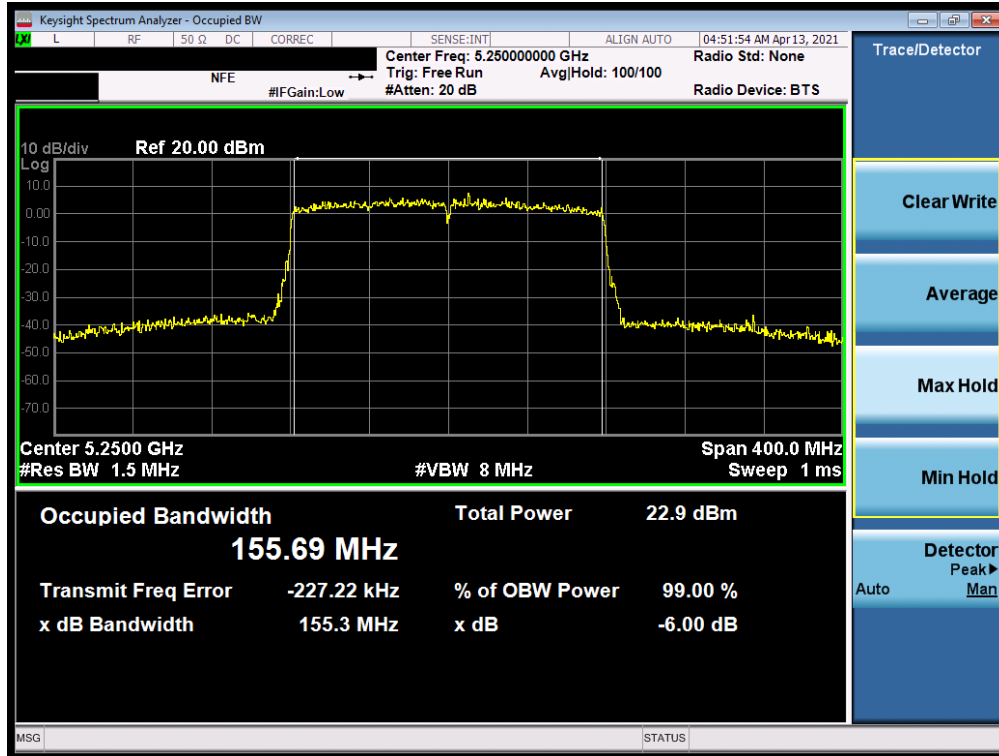
Plot 7-55. 26dB Bandwidth Plot SISO ANT1 (160MHz BW 802.11ax (UNII Band 2C) – Ch. 114)
