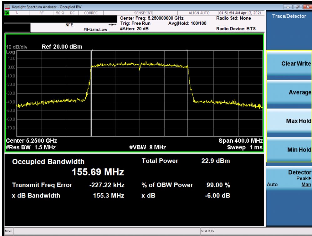
Plot 7-17. 26dB Bandwidth Plot SISO ANT1 (160MHz BW 802.11ax (UNII Band 1/2A) – Ch. 50)
