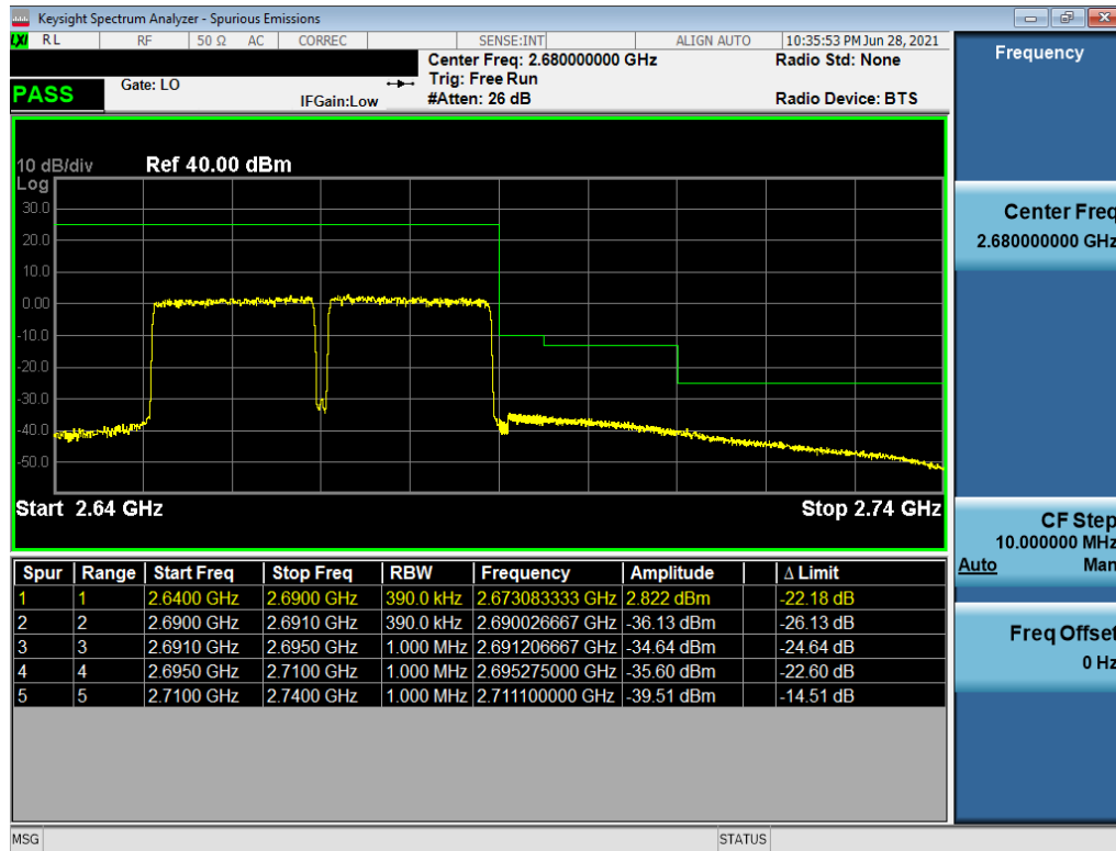
Plot 7-40. Upper ACP Plot (ULCA LTE B41(PC3) - 20MHz QPSK - Full RB - Ant1)
