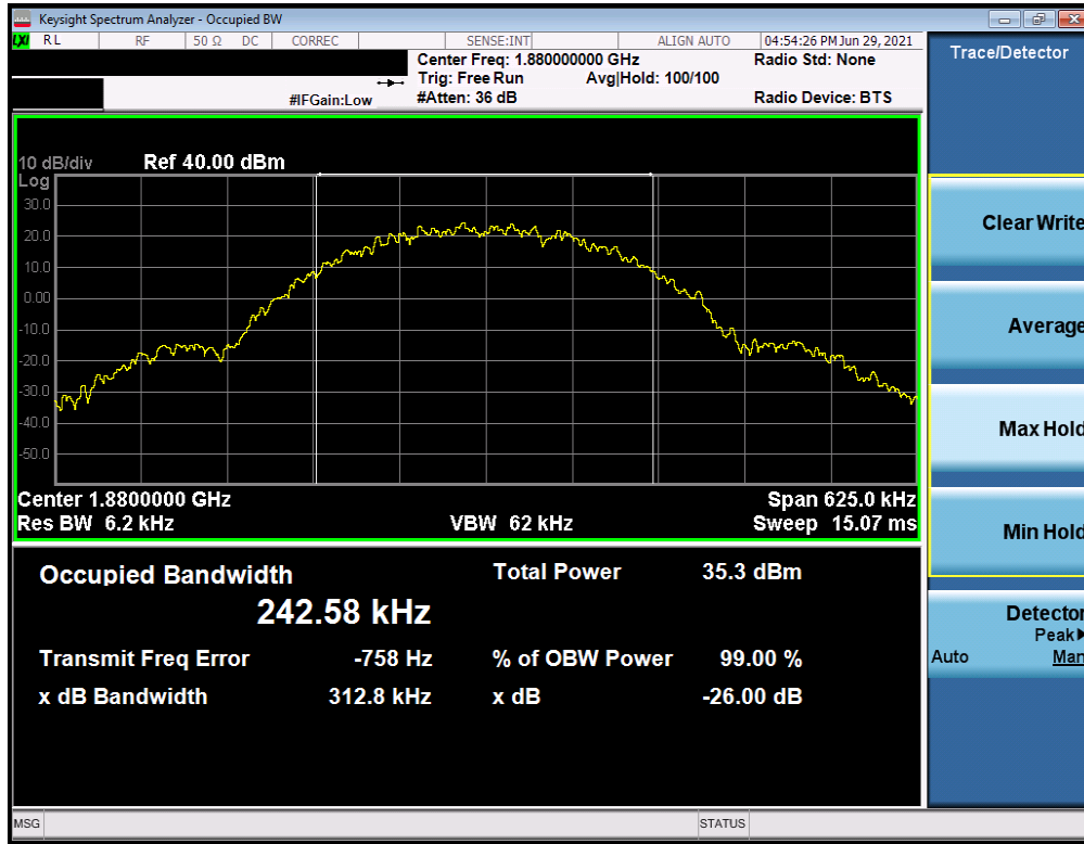
Plot 7-1. Occupied Bandwidth Plot (GPRS, Ch. 661)
