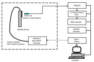
Figure 4-12 Audio Magnetic Field Test Setup
