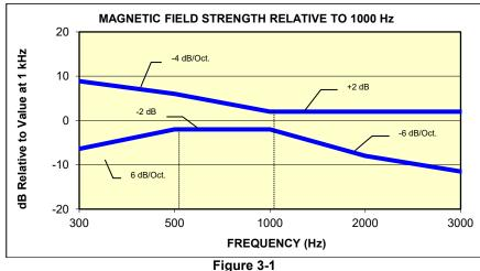
Magnetic field frequency response for Wireless Devices with an axial field ≤-15 dB(A/m) at 1 kHz
