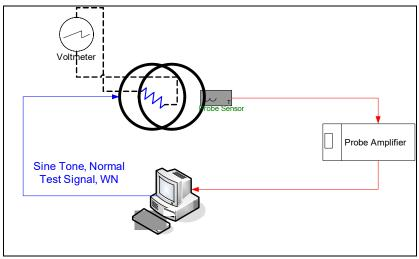
Figure 4-1 Validation Setup with Helmholtz Coil
