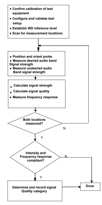
Figure 4-13 C63.19 T-Coil Signal Test Process
