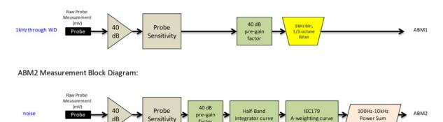
Figure 4-5 Magnetic Measurement Processing Steps
