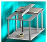
Figure 4-3 RF Near-Field Scanner
