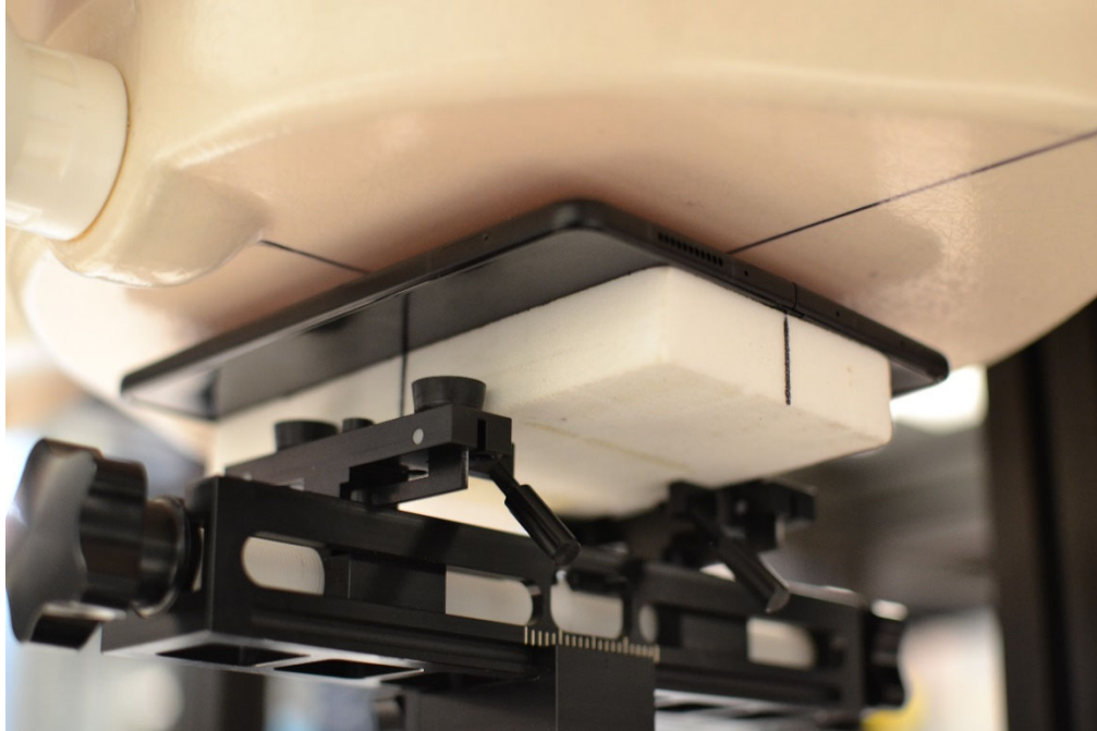
SAR Test Setup Photo 11– Open Configuration (UMPC), UMPC Body, Back Side, 10 mm
