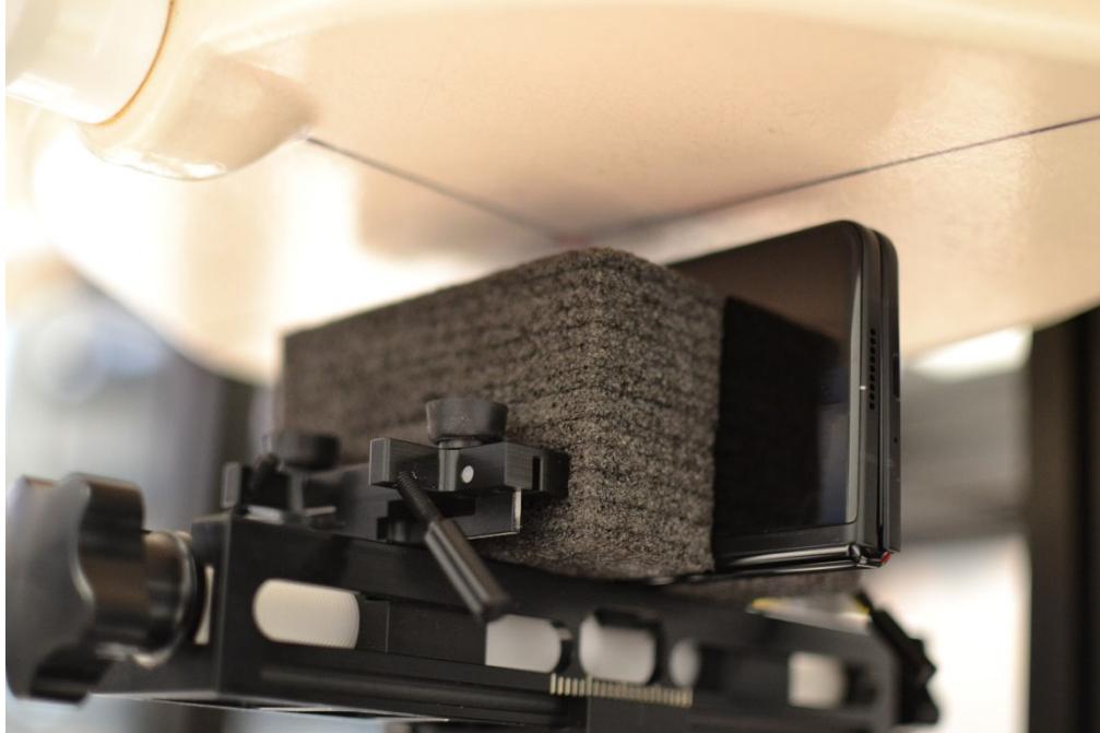
SAR Test Setup Photo 9– Closed Configuration (Handset), Hotspot, Right Edge, 10 mm
