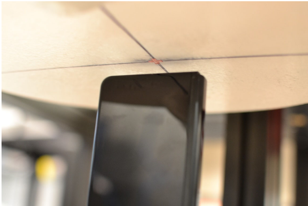
SAR Test Setup Photo 8– Closed Configuration (Handset), Hotspot, Bottom Edge, 10 mm
