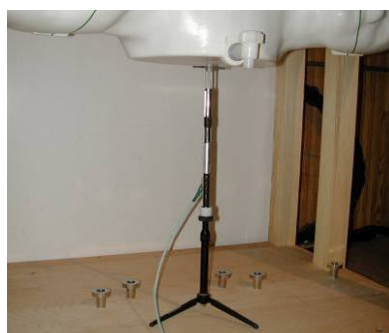
Figure 4-2 System Verification Setup Photo
