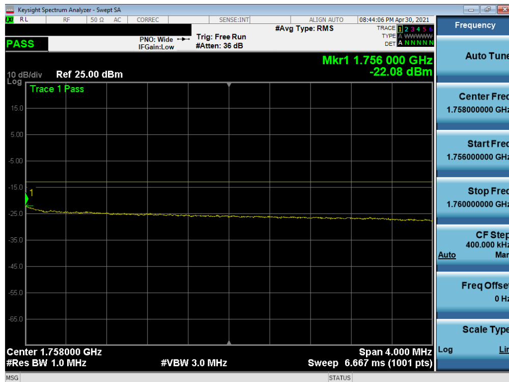
Plot 7-106. Upper Extended Band Edge Plot (LTE Band 4 - 10MHz QPSK – Full RB)
