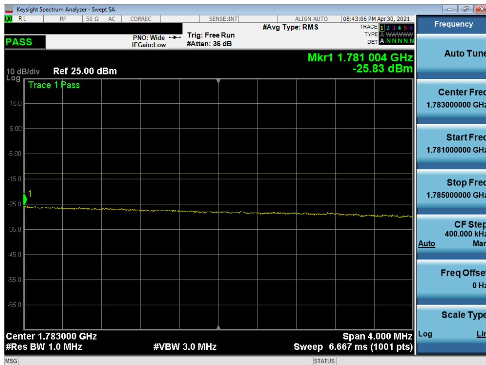
Plot 7-102. Upper Extended Band Edge Plot (LTE Band 66 - 15MHz QPSK – Full RB)
