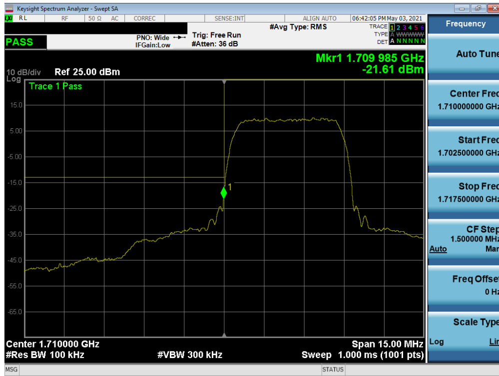
Plot 7-135. Lower Band Edge Plot (WCDMA AWS – Ch. 1312)
