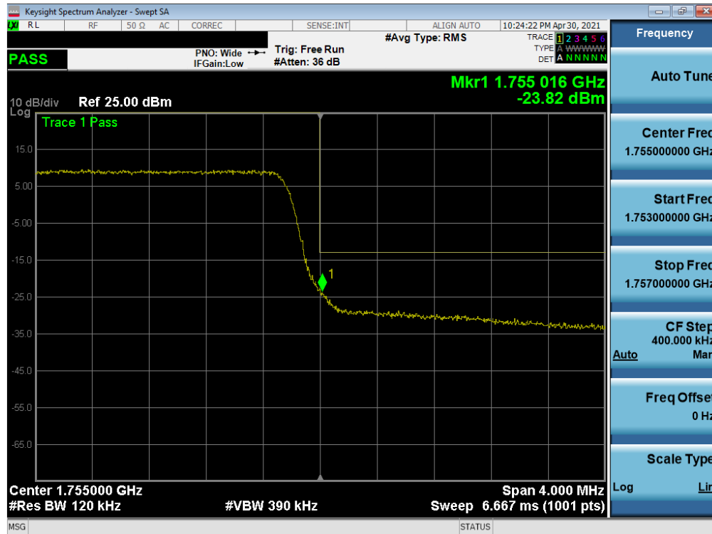
Plot 7-111. Upper Band Edge Plot (LTE Band 4 - 5MHz QPSK – Full RB)
