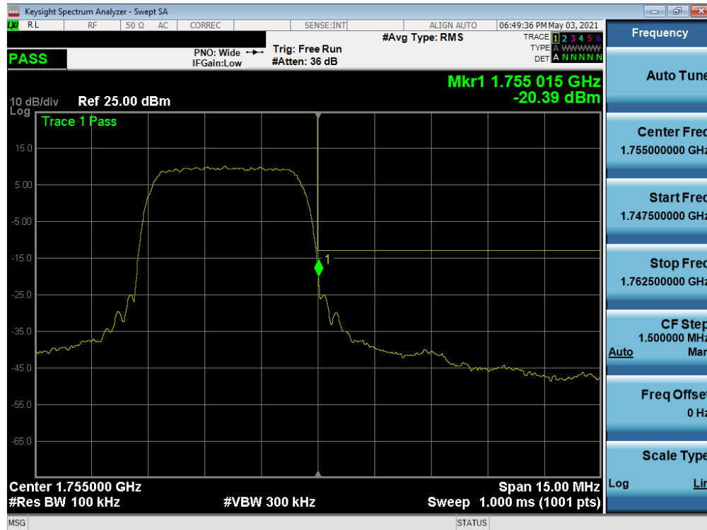
Plot 7-137. Upper Band Edge Plot (WCDMA AWS – Ch. 1513)
