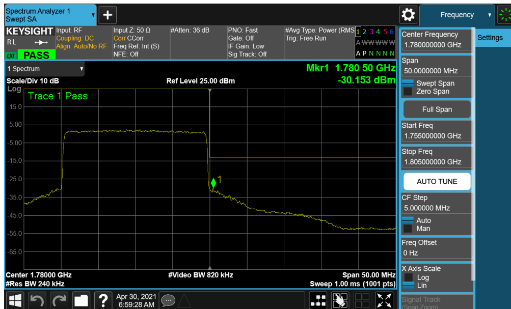
Plot 7-128. Upper Band Edge Plot (NR Band n66 – 20.0MHz - Full RB)
