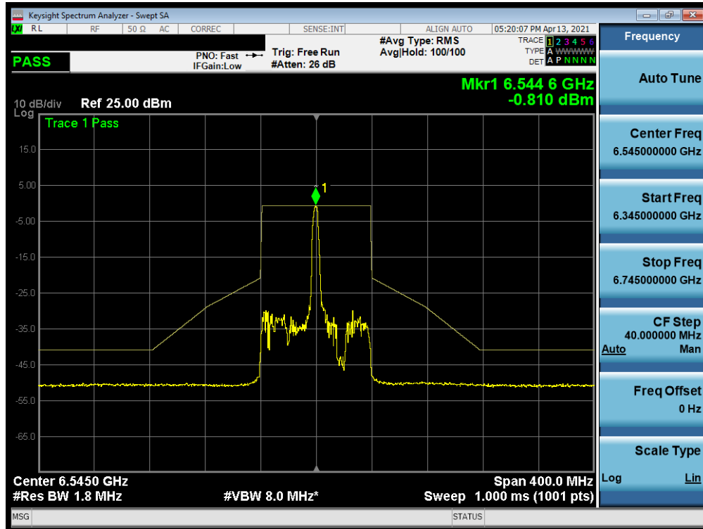
Plot 7-385. In-Band Emission Plot MIMO ANT2 (80MHz BW 802.11ax (26 Tones) (UNII Band 7) – Ch. 119)
