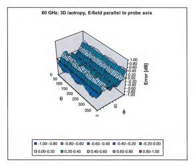
Probe isotropy for  $E_{tot}$ : probe rotated  $\varphi = 0^{\circ}$  to 360°, tilted from field propagation direction  $\overline{k}$ Parallel to the field propagation ( $\psi = 0^{\circ} - 90^{\circ}$ ) at 30 GHz: deviation within ± 0.47 dB Parallel to the field propagation ( $\psi = 0^{\circ} - 90^{\circ}$ ) at 60 GHz: deviation within ± 0.49 dB
