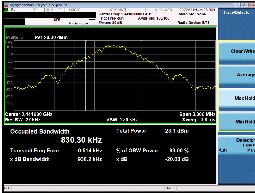
Plot 7-2. 20dB Bandwidth Plot (Bluetooth, 1Mbps – Ch. 39) Antenna 0
