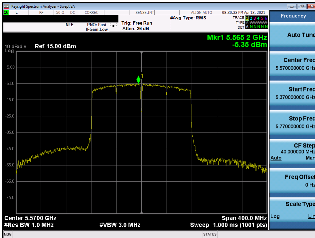
Plot 7-334. Power Spectral Density Plot MIMO ANT1 (160MHz BW 802.11ac (UNII Band 2C) – Ch. 114)
