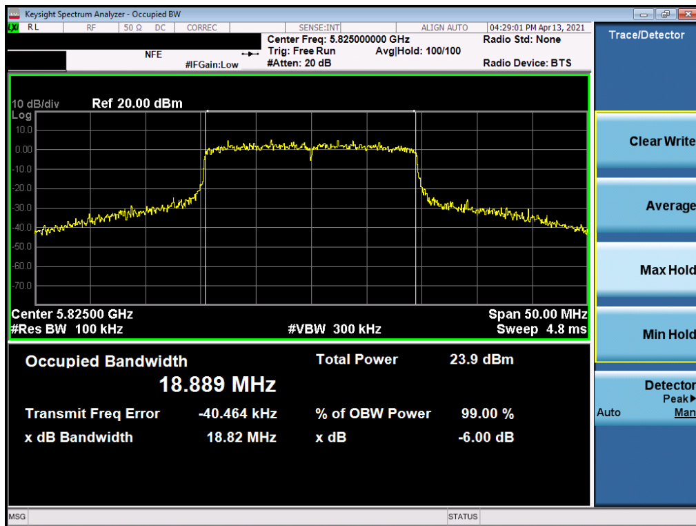
Plot 7-189. 6dB Bandwidth Plot MIMO ANT 1 (20MHz 802.11ax (UNII Band 3) – Ch. 165)
