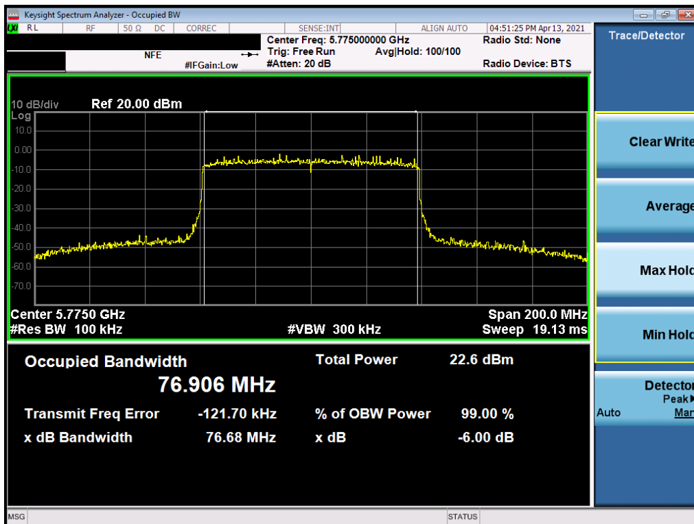
Plot 7-195. 6dB Bandwidth Plot MIMO ANT 1 (80MHz 802.11ax (UNII Band 3) – Ch. 155)
