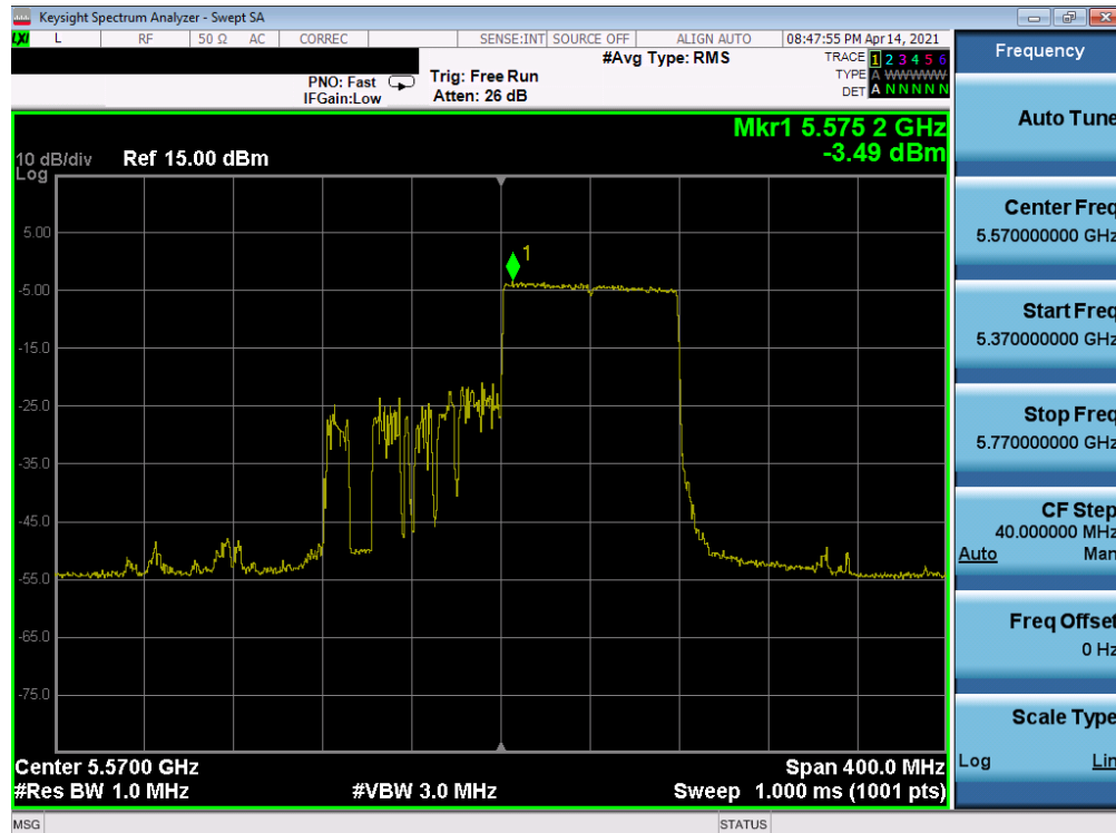
Plot 7-242. Power Spectral Density Plot MIMO ANT2 (160MHz BW(U) 802.11ax – Full Tones (UNII Band 2C) – Ch. 114)
