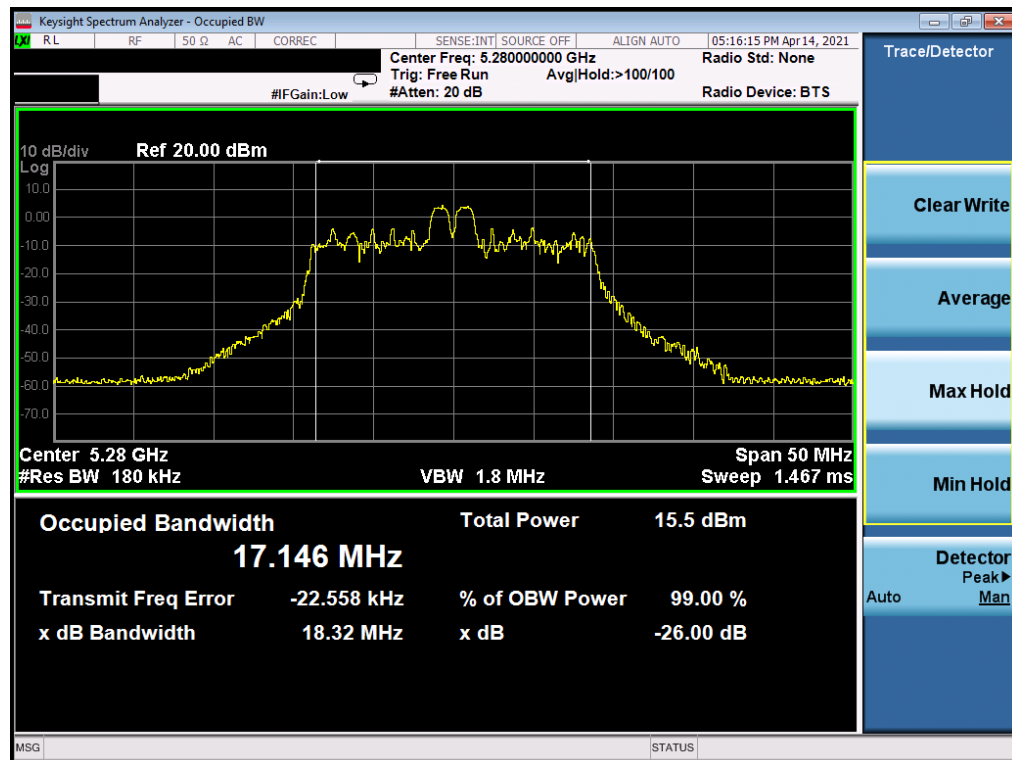
Plot 7-35. 26dB Bandwidth Plot MIMO ANT2 (20MHz BW 802.11ax – 26 Tones (UNII Band 2A) – Ch. 56)
