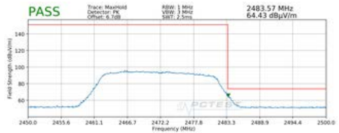
Plot 7-180. Radiated Restricted Upper Band Edge Measurement MIMO (Peak) – OPEN
