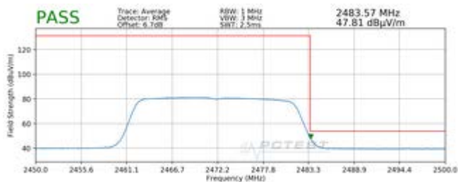
Plot 7-169. Radiated Restricted Upper Band Edge Measurement SISO ANT2 (Average) – OPEN
