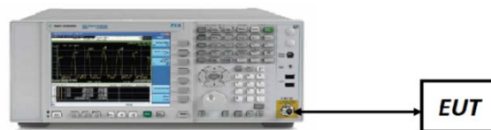
Figure 7-5. Test Instrument & Measurement Setup
