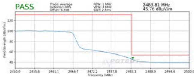
Plot 7-173. Radiated Restricted Upper Band Edge Measurement MIMO (Average) – OPEN
