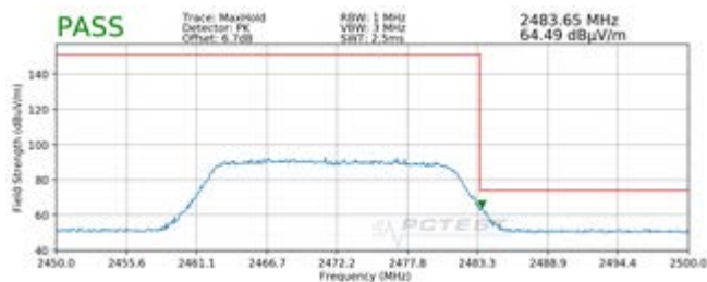
Plot 7-170. Radiated Restricted Upper Band Edge Measurement SISO ANT2 (Peak) – OPEN
