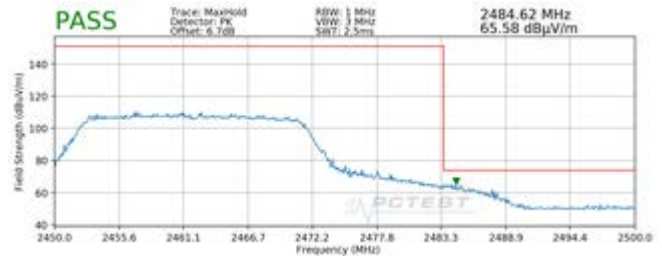
Plot 7-166. Radiated Restricted Upper Band Edge Measurement SISO ANT2 (Peak) – OPEN
