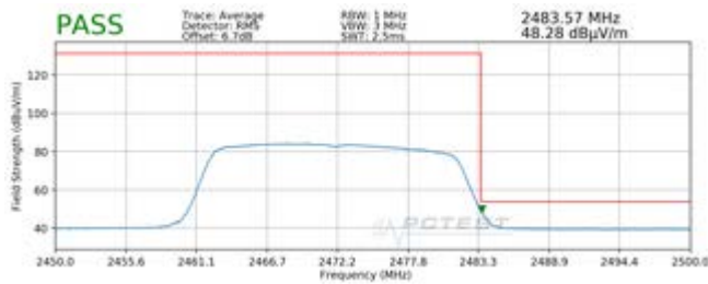
Plot 7-179. Radiated Restricted Upper Band Edge Measurement MIMO (Average) – OPEN
