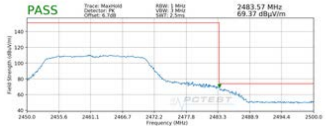
Plot 7-176. Radiated Restricted Upper Band Edge Measurement MIMO (Peak) – OPEN
