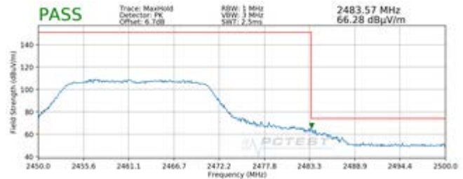
Plot 7-182. Radiated Restricted Band Edge Measurement MIMO with WCP (Peak) – OPEN
