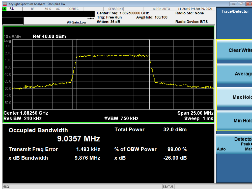
Plot 7-5. Occupied Bandwidth Plot (LTE Band 25/2 - 10MHz QPSK - Full RB)
