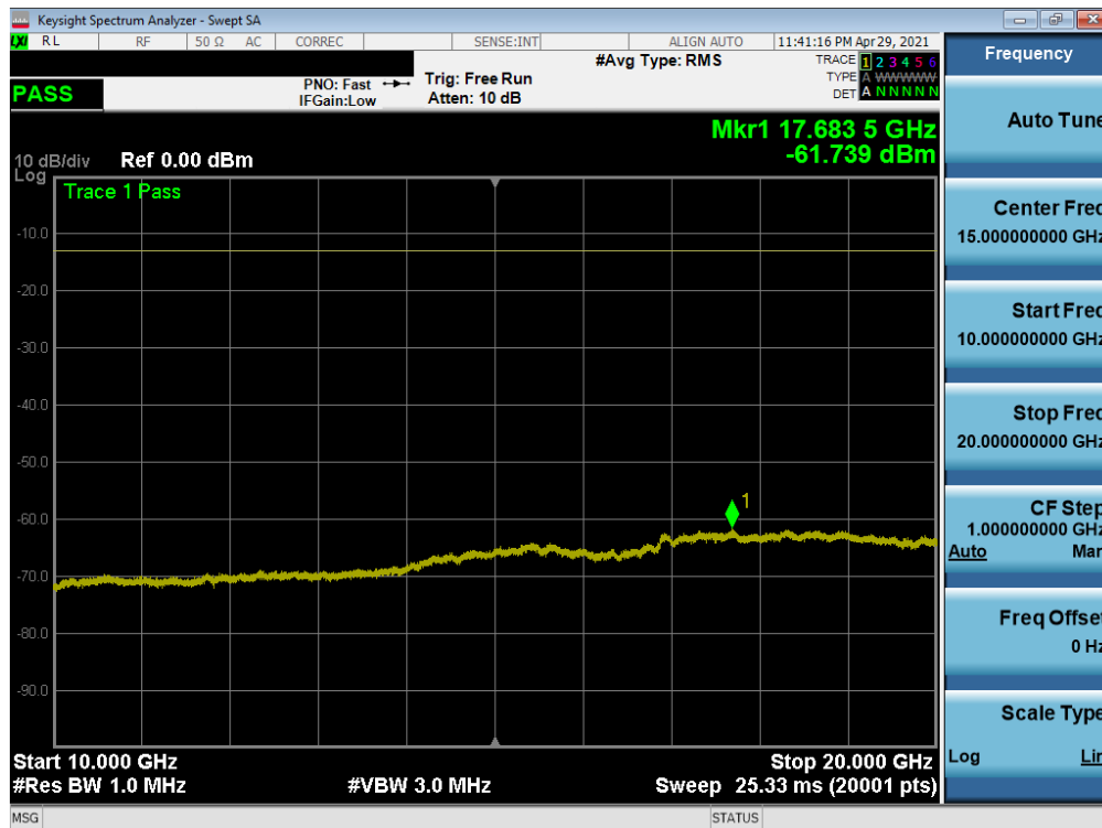
Plot 7-21. Conducted Spurious Plot (LTE Band 25/2 - 20MHz QPSK - 1RB - Mid Channel)
