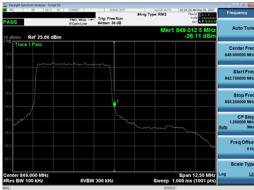
Plot 7-83. Upper Band Edge Plot (NR Band n5 – 5.0MHz DFT-s-OFDM-QPSK - Full RB)
