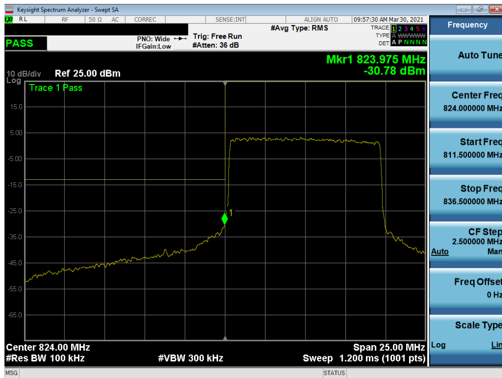
Plot 7-80. Lower Band Edge Plot (NR Band n5 – 10.0MHz DFT-s-OFDM-QPSK - Full RB)
