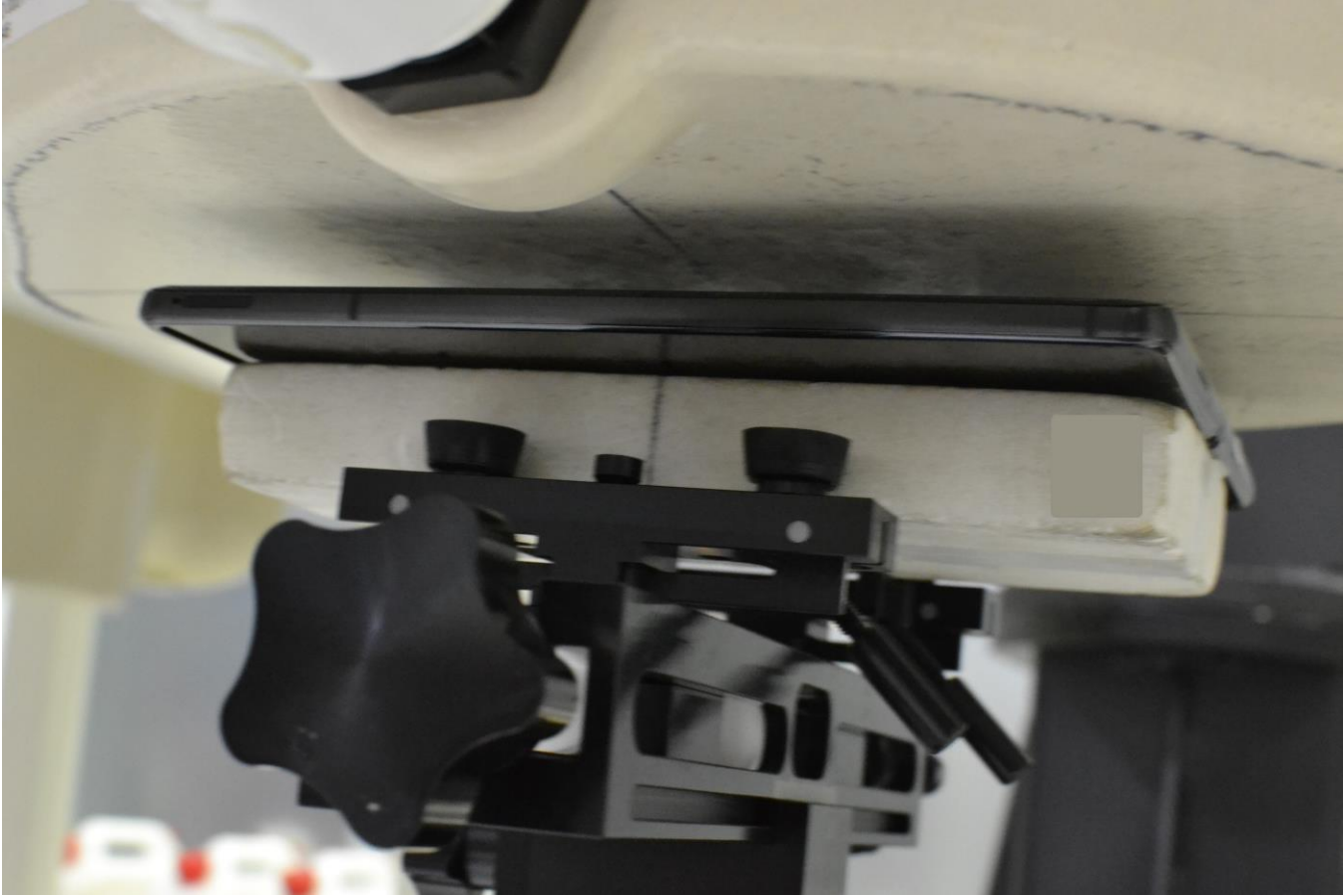
Test Setup Photo 7 – Open, Back Side 12mm SAR
