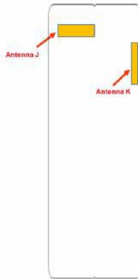
Figure 1: Location of mmW antenna modules looking from front of the DUT – closed
