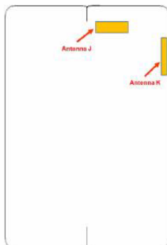
Figure 2: Location of mmW antenna modules looking from front of the DUT - open
