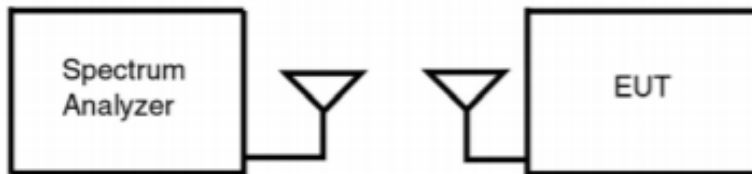
Figure 7-1. Test Instrument and Measurement Setup
