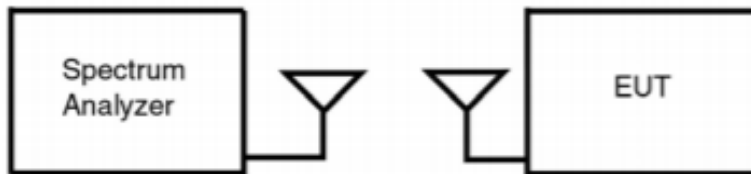
Figure 7-2. Test Instrument and Measurement Setup
