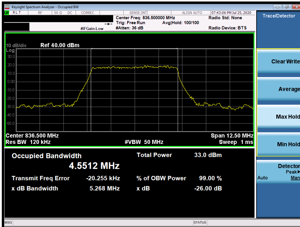
Plot 7-96. Occupied Bandwidth Plot (NR Band n5 - 5.0MHz DFT-s-OFDM BPSK - Full RB)
