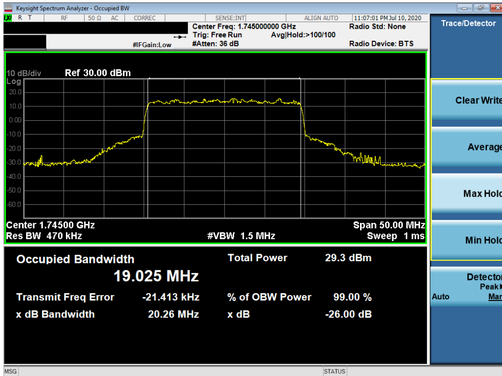
Plot 7-126. Occupied Bandwidth Plot (NR Band n66 - 20.0MHz CP-OFDM QPSK - Full RB)
