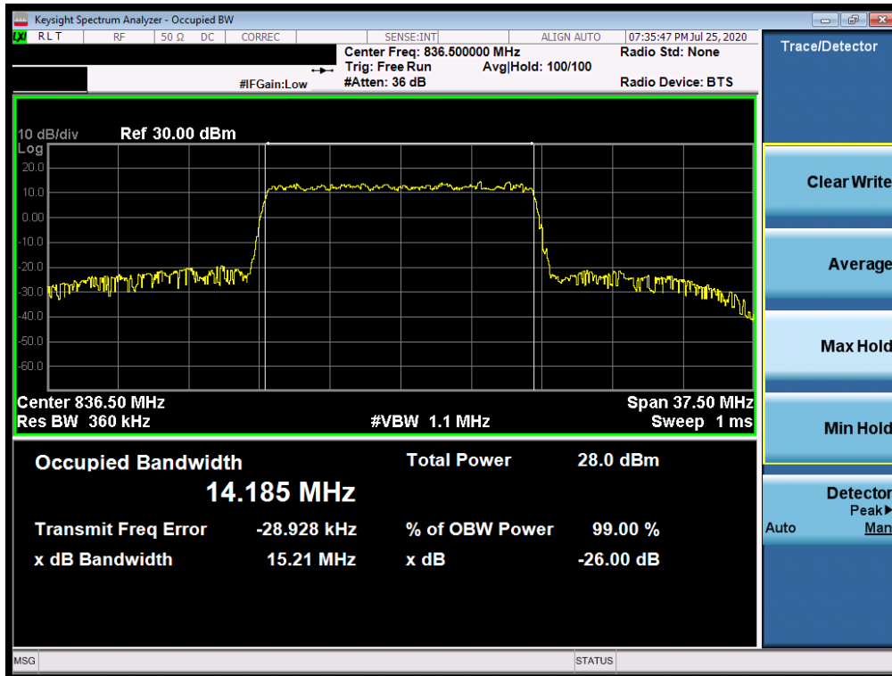
Plot 7-90. Occupied Bandwidth Plot (NR Band n5 - 15.0MHz CP-OFDM 256QAM - Full RB)
