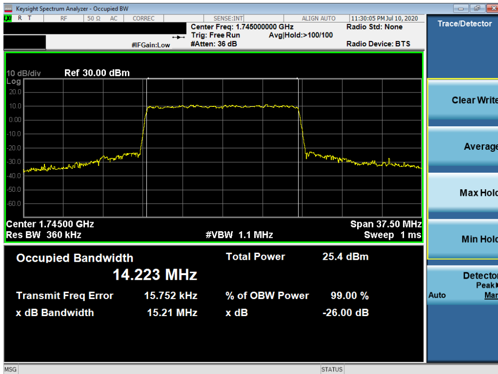
Plot 7-134. Occupied Bandwidth Plot (NR Band n66 - 15.0MHz CP-OFDM 256QAM - Full RB)
