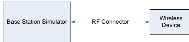
Figure 9-1 Power Measurement Setup
