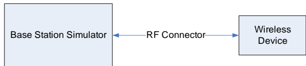
Figure 9-4 Power Measurement Setup
