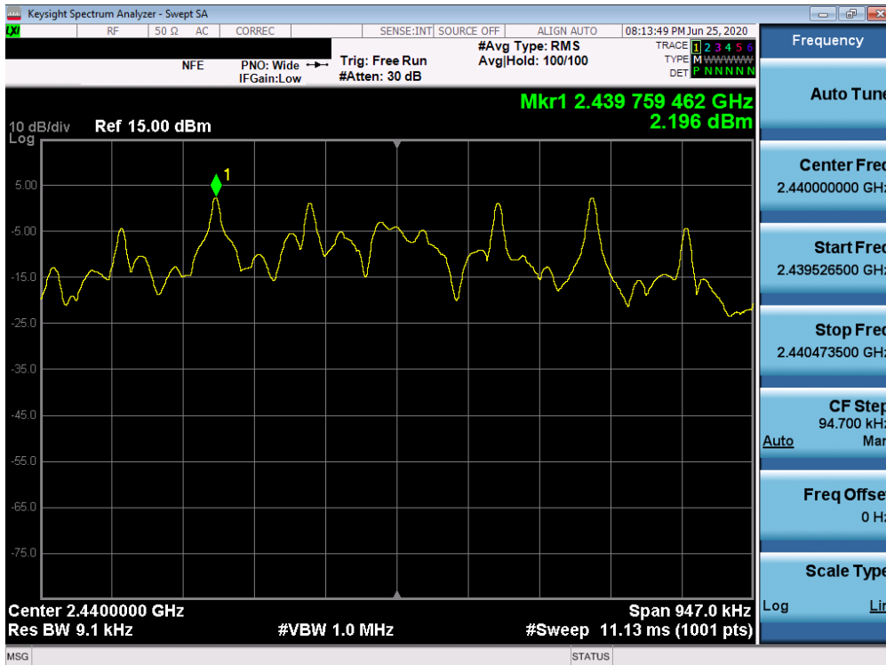
Plot 7-32. Power Spectral Density Plot (Bluetooth (LE), 1Mbps – Ch. 19)
