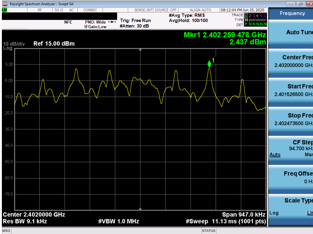
Plot 7-31. Power Spectral Density Plot (Bluetooth (LE), 1Mbps – Ch. 0)
