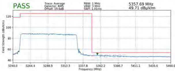
Plot 7-311. Radiated Upper Band Edge Plot SISO ANT1 (Average – UNII Band 2A)
