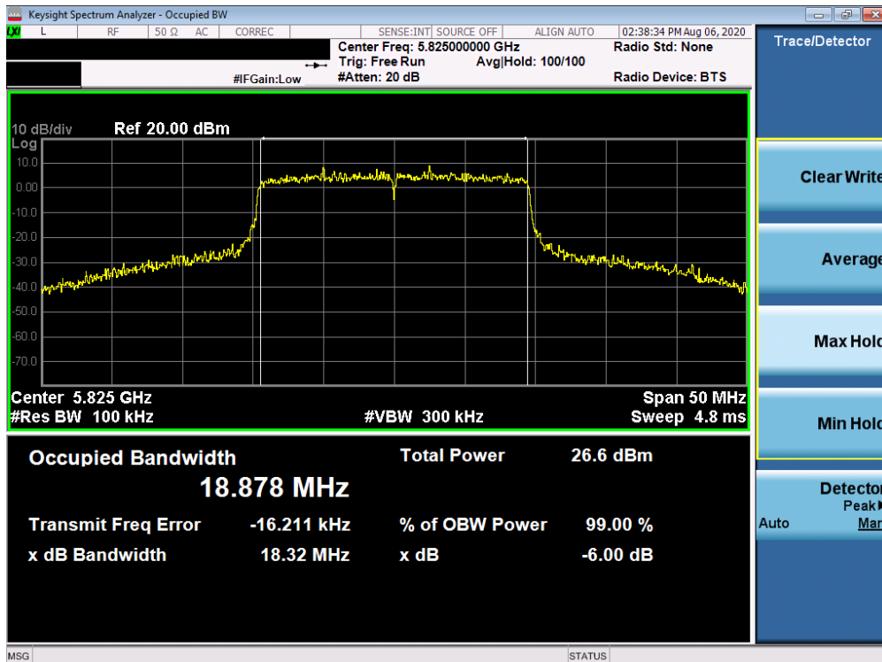
Plot 7-129. 6dB Bandwidth Plot SISO ANT2 (20MHz BW 802.11ax (UNII Band 3) – Ch. 165)
