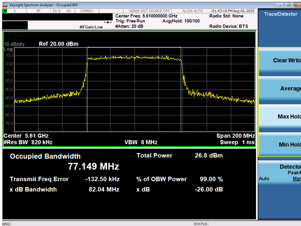
Plot 7-101. 26dB Bandwidth Plot SISO ANT2 (80MHz BW 802.11ax (UNII Band 2C) – Ch. 122)
