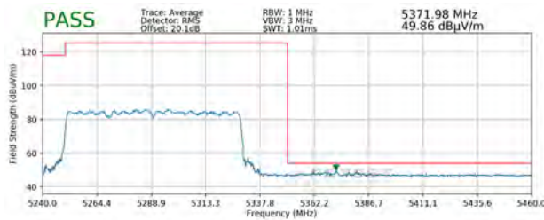
Plot 7-311. Radiated Upper Band Edge Plot MIMO (Average – UNII Band 2A – 996 Tones)
