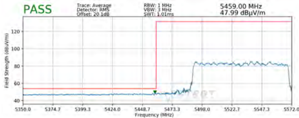
Plot 7-313. Radiated Lower Band Edge Plot MIMO (Average – UNII Band 2C – 996 Tones)
