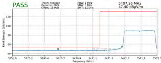
Plot 7-264. Radiated Lower Band Edge Plot SISO ANT1 (Average – UNII Band 2C – 484 Tones)
