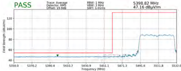
Plot 7-306. Radiated Lower Band Edge Plot MIMO (Average – UNII Band 2C – 484 Tones)
