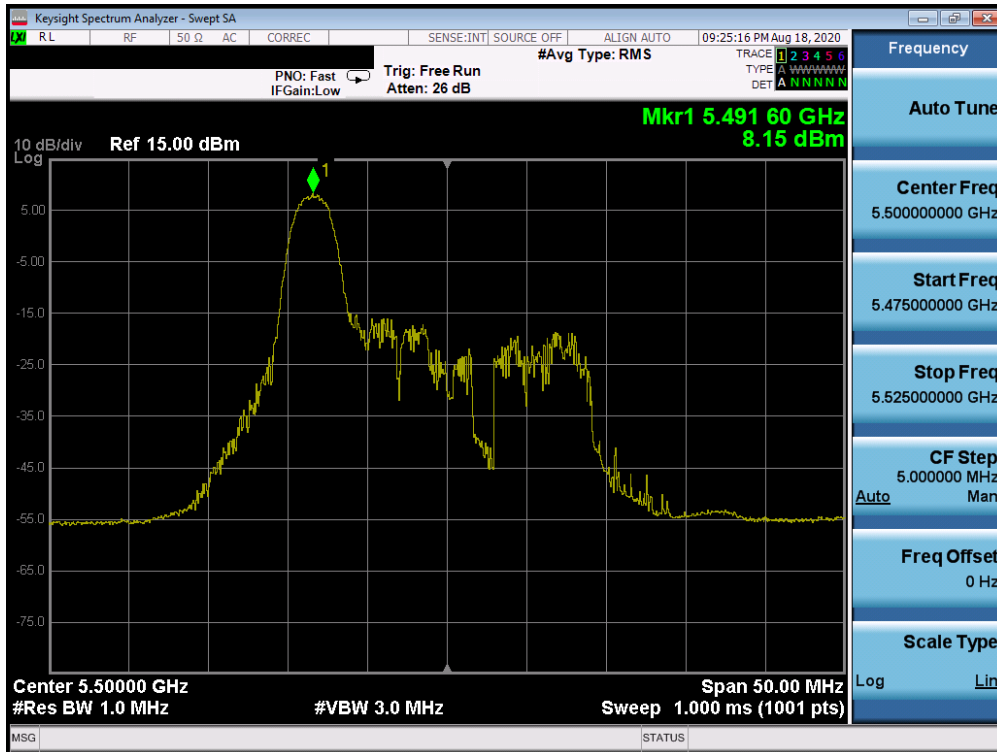
Plot 7-121. Power Spectral Density Plot SISO ANT1 (20MHz BW 802.11ax – 26 Tones (UNII Band 2C) – Ch. 100)
