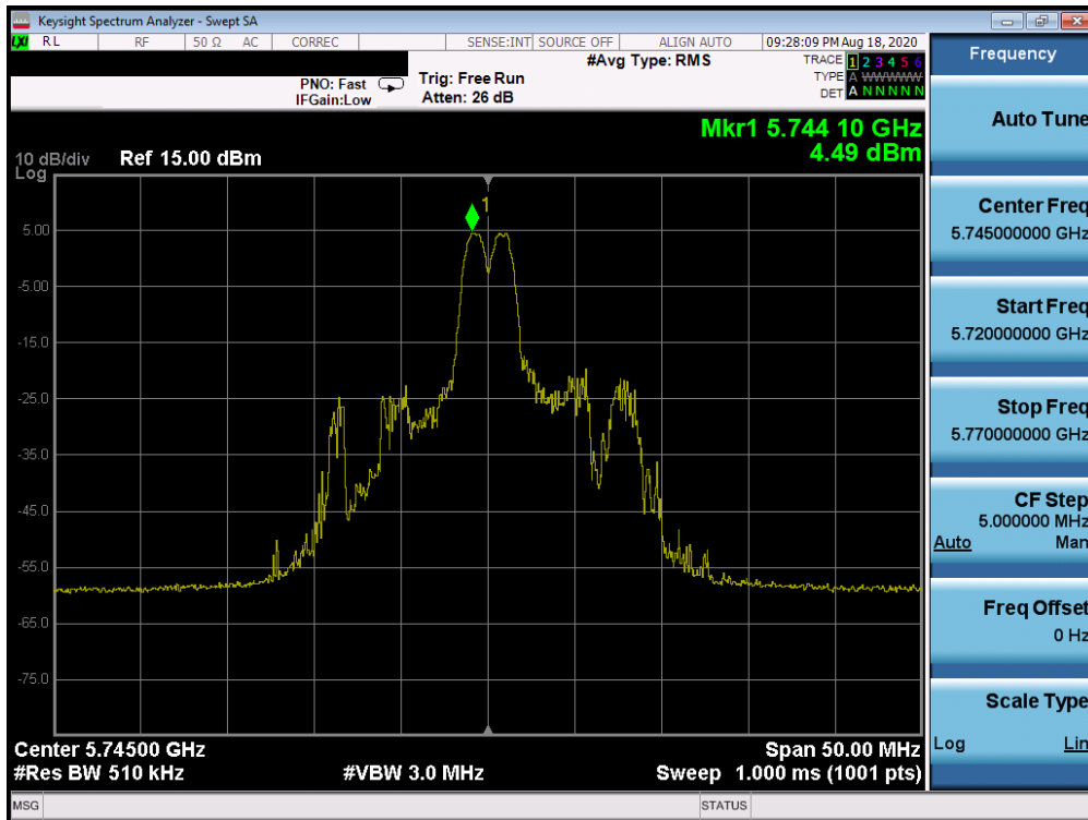
Plot 7-130. Power Spectral Density Plot SISO ANT1 (20MHz BW 802.11ax – 26 Tones (UNII Band 3) – Ch. 149)
