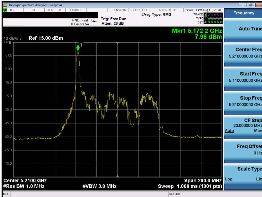
Plot 7-114. Power Spectral Density Plot SISO ANT1 (80MHz BW 802.11ax – 26 Tones (UNII Band 1) – Ch. 42)
