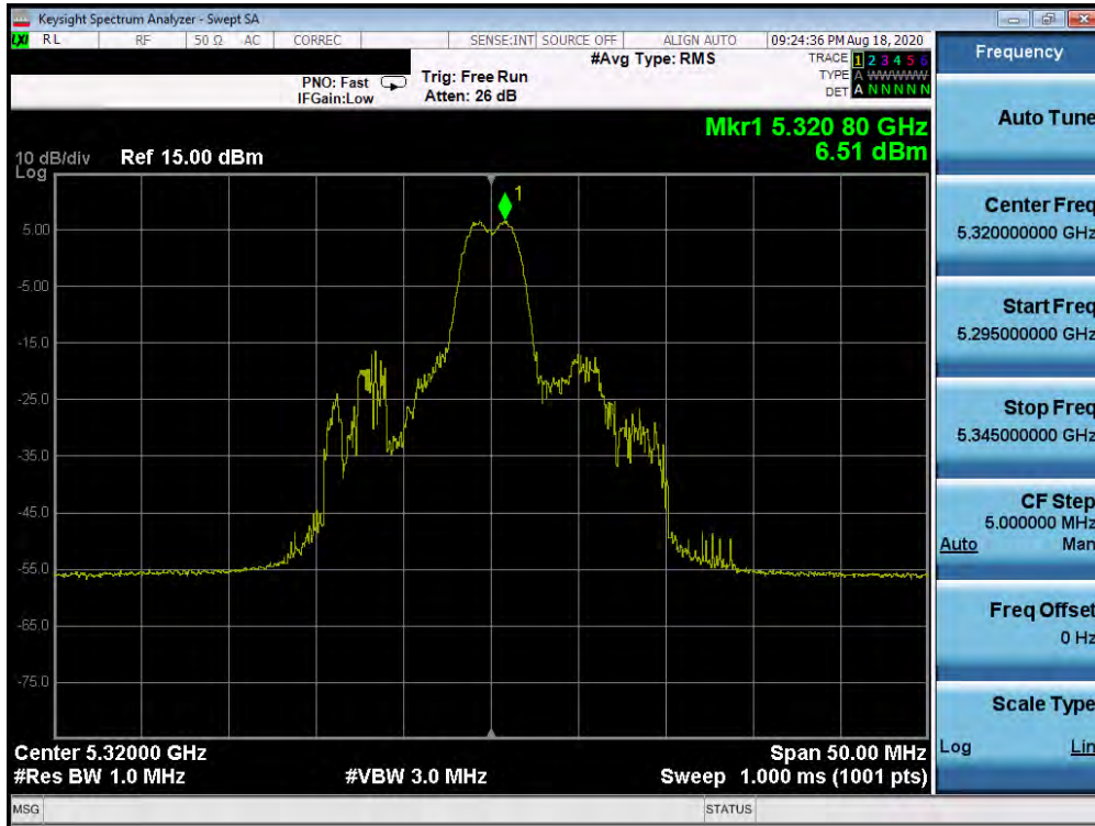
Plot 7-117. Power Spectral Density Plot SISO ANT1 (20MHz BW 802.11ax – 26 Tones (UNII Band 2A) – Ch. 64)
