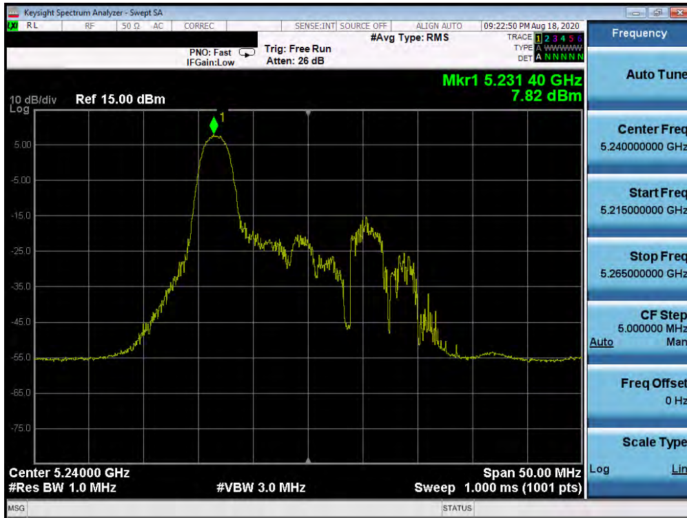
Plot 7-111. Power Spectral Density Plot SISO ANT1 (20MHz BW 802.11ax – 26 Tones (UNII Band 1) – Ch. 48)
