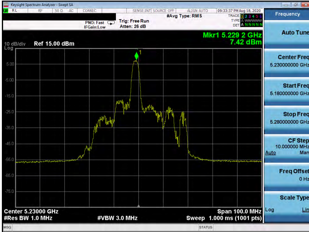
Plot 7-113. Power Spectral Density Plot SISO ANT1 (40MHz BW 802.11ax – 26 Tones (UNII Band 1) – Ch. 46)
