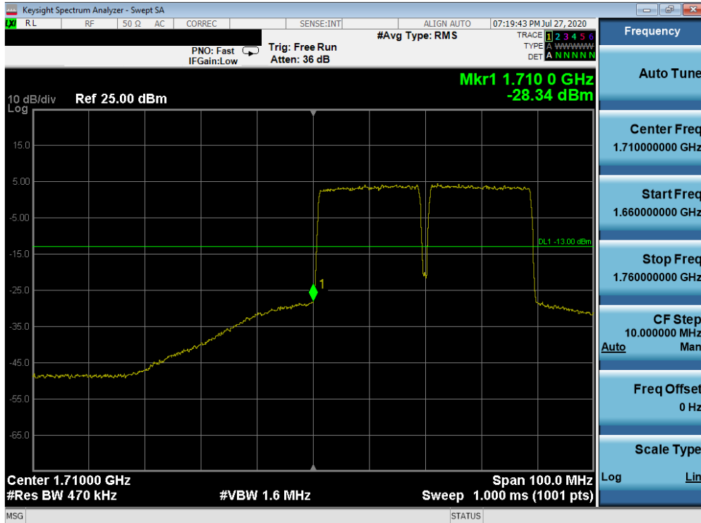
Plot 7-694. Lower Band Edge Plot (Band 66 QPSK – PCC:20 MHz SCC:20 MHz – Full RB)
