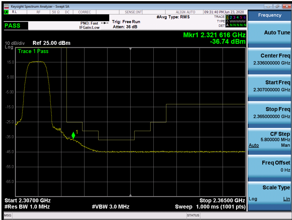
Plot 7-541. Upper Extended Band Edge Plot (Band 30 - 5.0MHz QPSK - Full RB Configuration)
