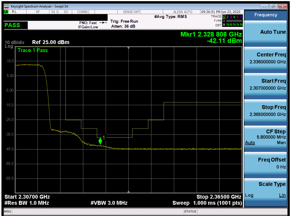
Plot 7-545. Upper Extended Band Edge Plot (Band 30 - 10.0MHz QPSK - Full RB Configuration)
