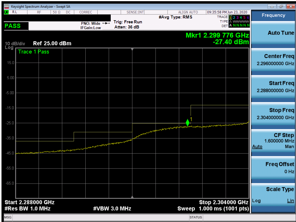
Plot 7-543. Lower Extended Band Edge Plot (Band 30 - 10.0MHz QPSK - Full RB Configuration)
