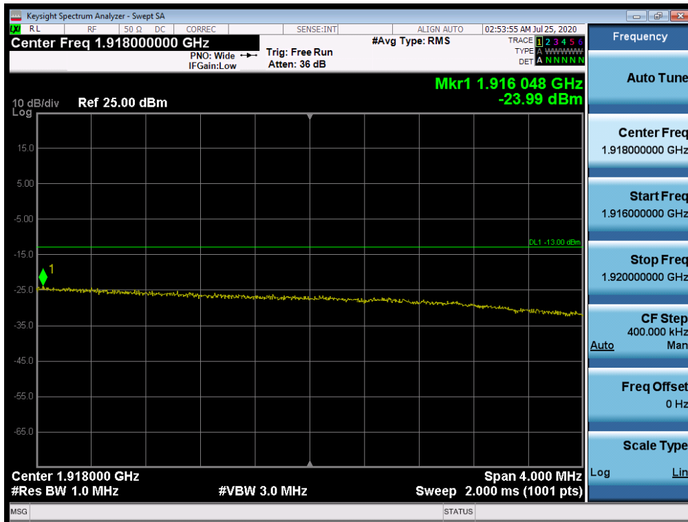
Plot 7-531. Upper Extended Band Edge Plot (NR Band n25 – 15.0MHz - Full RB)
