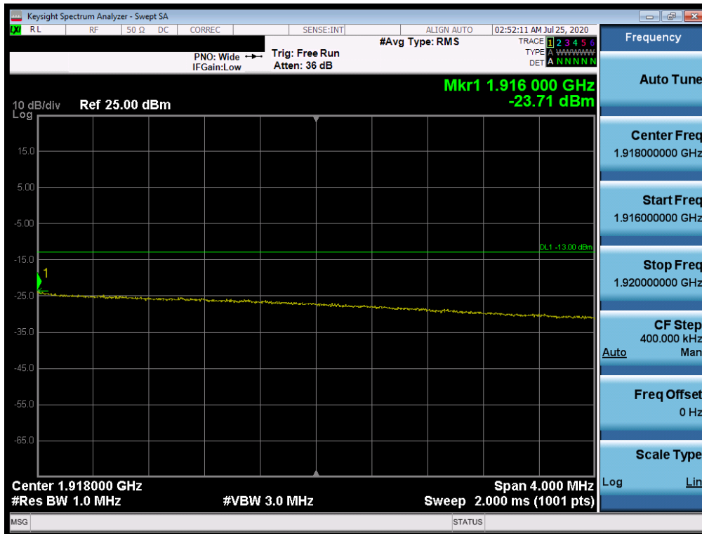
Plot 7-537. Upper Extended Band Edge Plot (NR Band n25 – 20.0MHz - Full RB)
