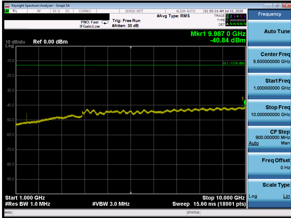
Plot 7-290. Conducted Spurious Plot (Band 12 - 10.0MHz QPSK - RB Size 1, RB Offset 0 - High Channel)
