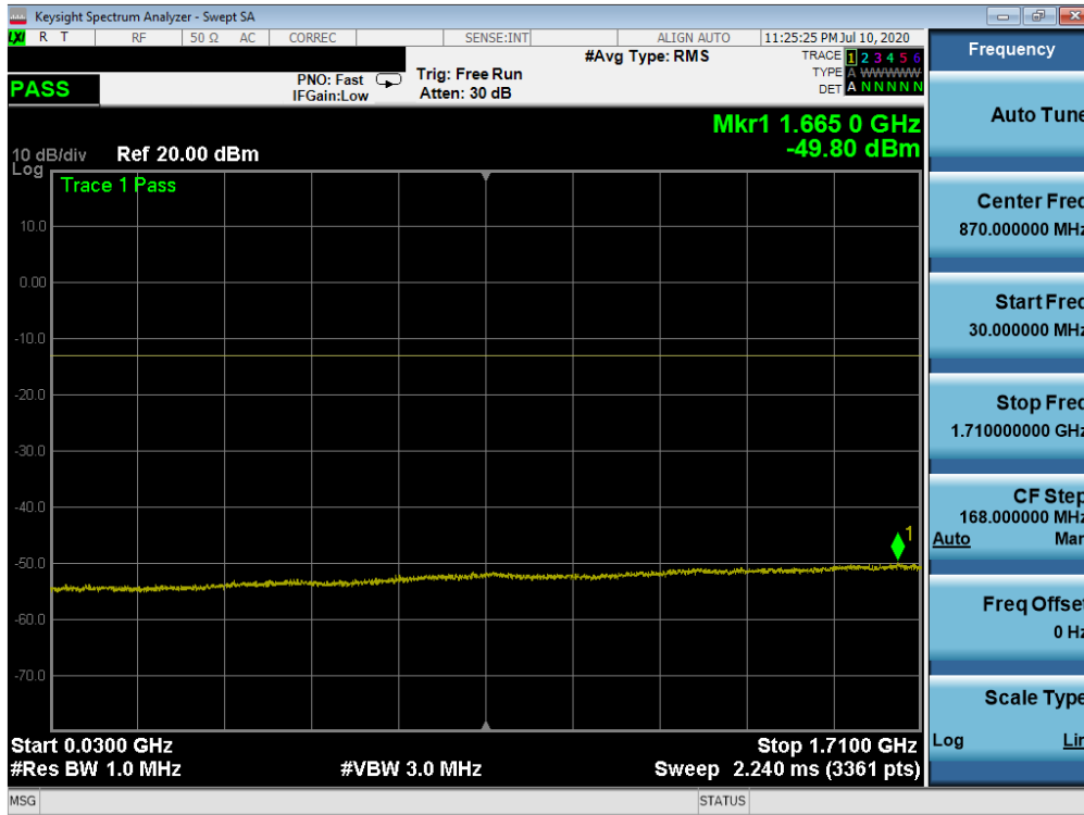
Plot 7-321. Conducted Spurious Plot (NR Band n66 -20.0MHz - RB Size 1, RB Offset 0 - Low Channel)
