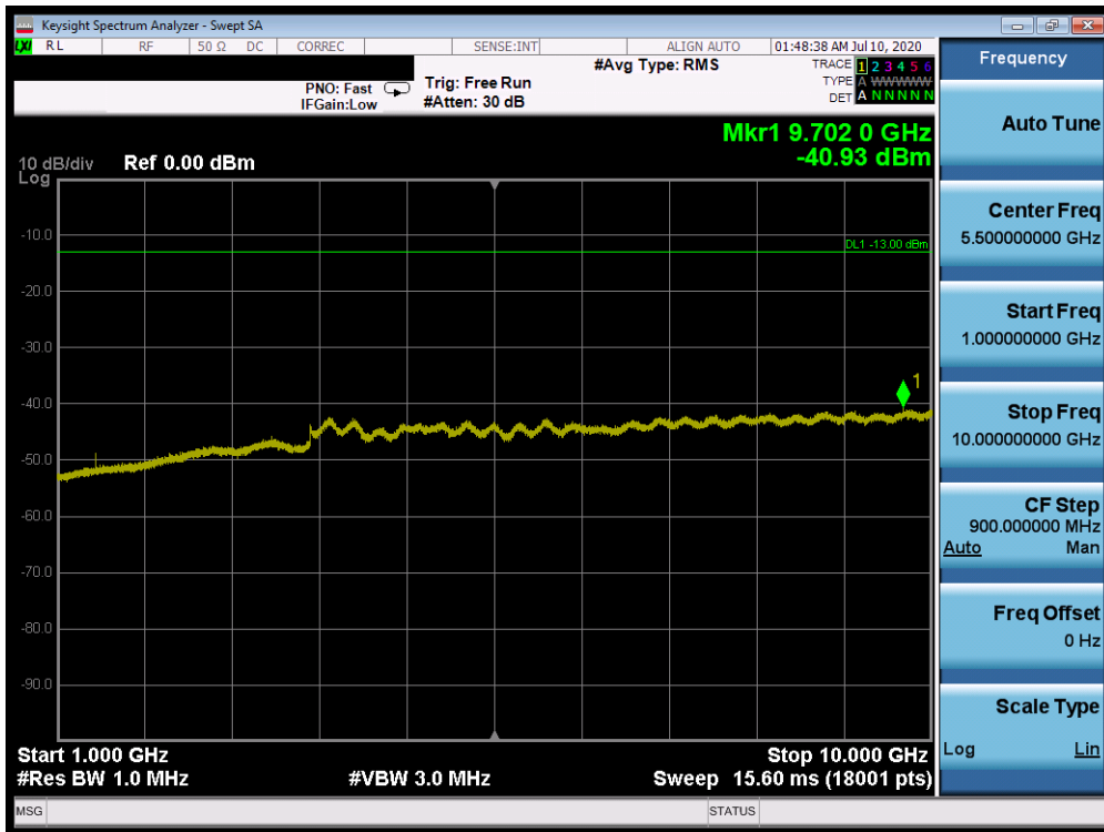
Plot 7-284. Conducted Spurious Plot (Band 12 - 10.0MHz QPSK - RB Size 1, RB Offset 0 - Low Channel)
