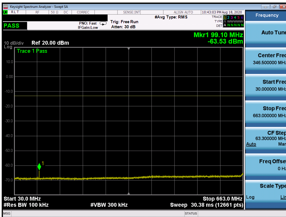
Plot 7-276. Conducted Spurious Plot (NR Band n71 - 20.0MHz - RB Size 1, RB Offset 0 - Mid Channel)
