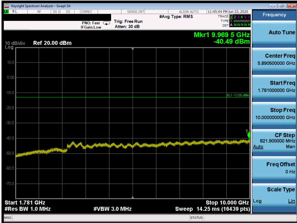
Plot 7-319. Conducted Spurious Plot (Band 66/4 - 20.0MHz QPSK - RB Size 1, RB Offset 0 - High Channel)
