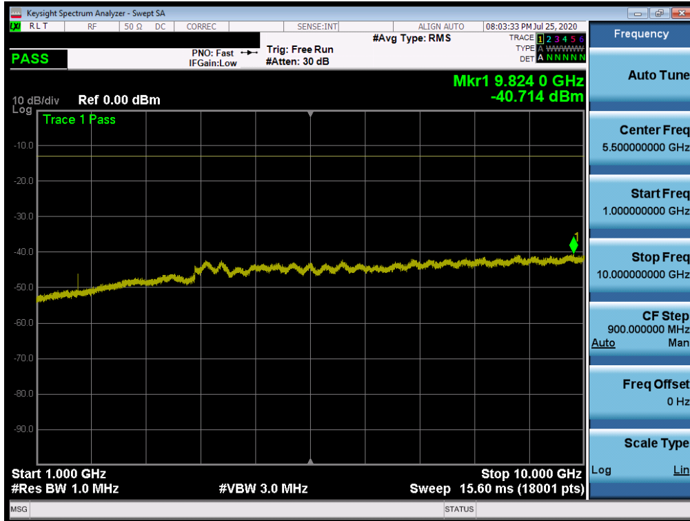
Plot 7-311. Conducted Spurious Plot (NR Band n5 - 20.0MHz - RB Size 1, RB Offset 0 - High Channel)
