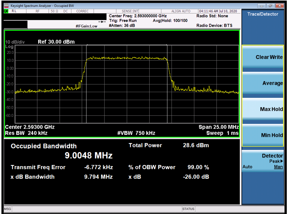
Plot 7-223. Occupied Bandwidth Plot (Band 41 (PC2) - 10.0MHz 64-QAM - Full RB Configuration)
