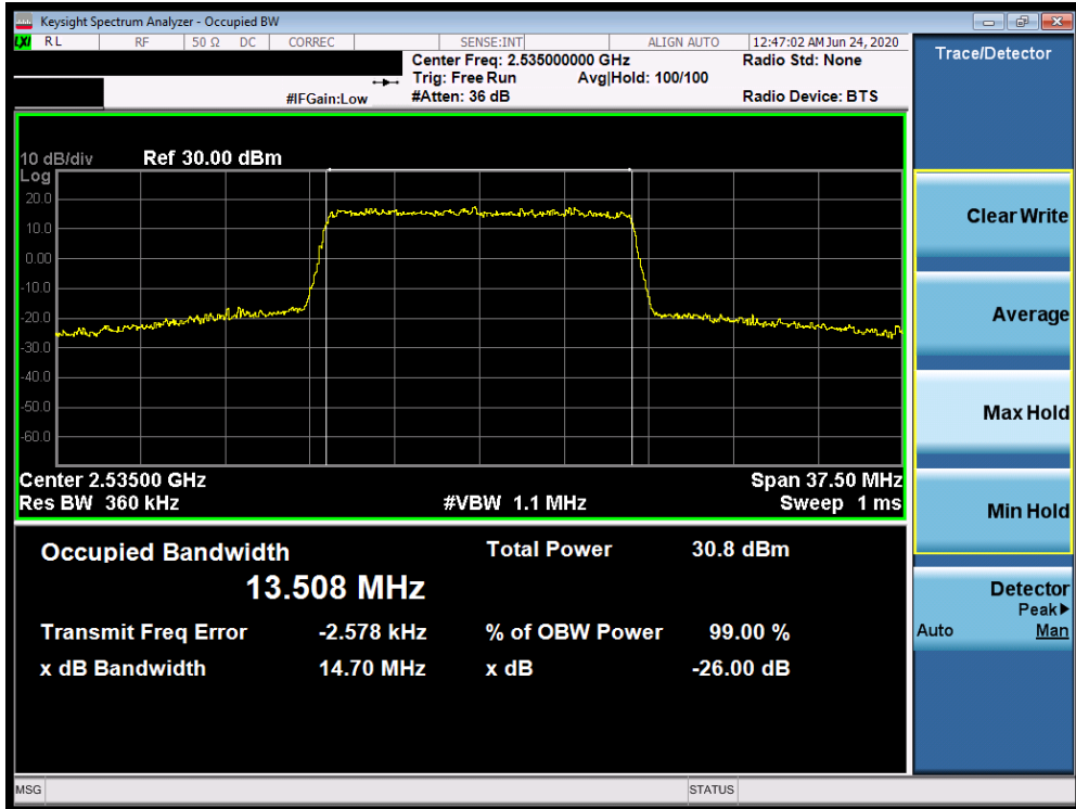
Plot 7-202. Occupied Bandwidth Plot (Band 7 - 15.0MHz 16-QAM - Full RB Configuration)
