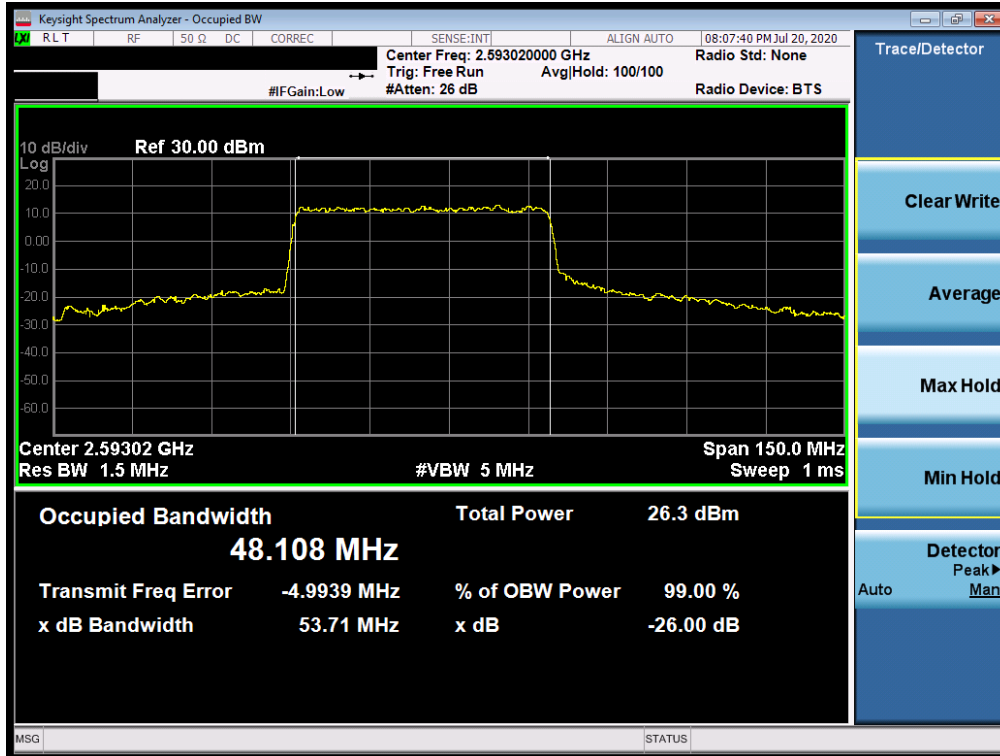
Plot 7-251. Occupied Bandwidth Plot (NR Band n41 - 50MHz CP-OFDM 16-QAM - Full RB)
