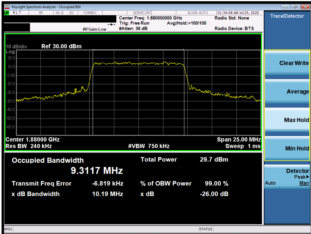
Plot 7-180. Occupied Bandwidth Plot (n25/2 10MHz QPSK-CP-OFDM - Full RB Configuration)
