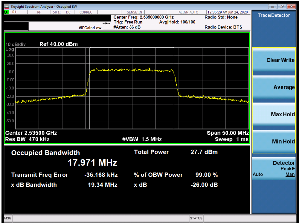
Plot 7-200. Occupied Bandwidth Plot (Band 7 - 20.0MHz 256-QAM - Full RB Configuration)
