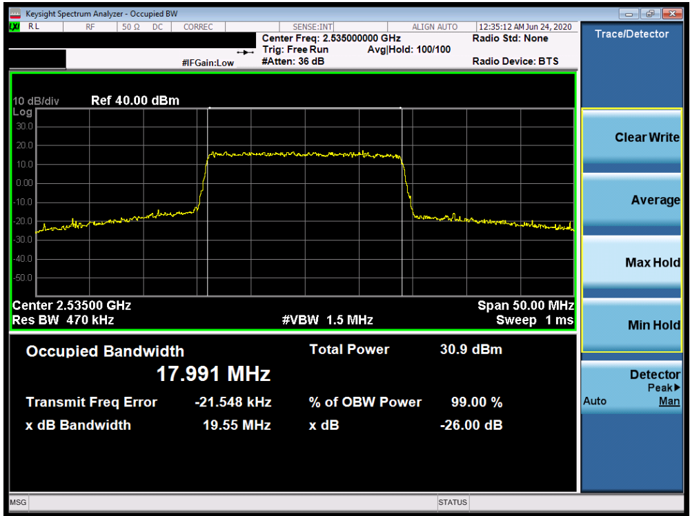
Plot 7-198. Occupied Bandwidth Plot (Band 7 - 20.0MHz 16-QAM - Full RB Configuration)
