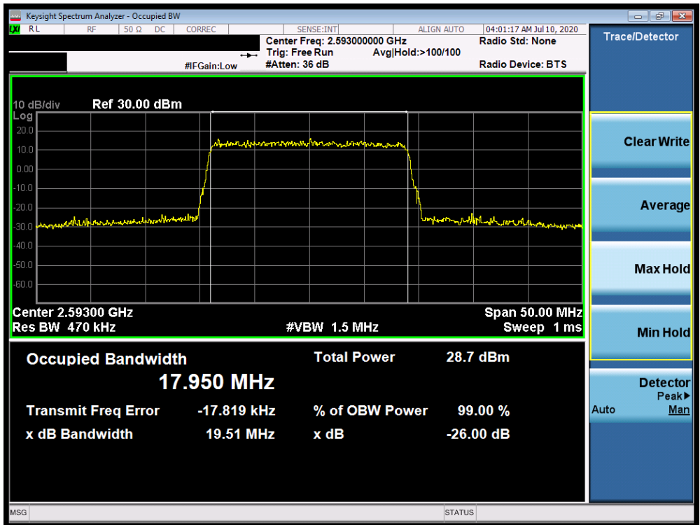
Plot 7-215. Occupied Bandwidth Plot (Band 41 (PC2) - 20.0MHz 64-QAM - Full RB Configuration)
