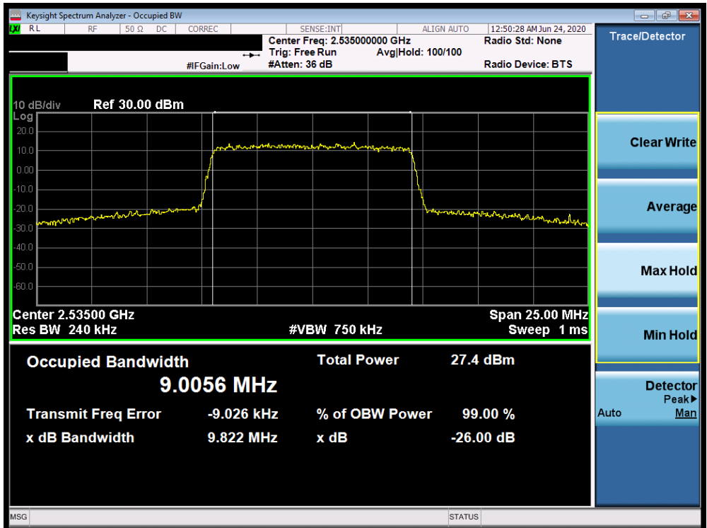
Plot 7-208. Occupied Bandwidth Plot (Band 7 - 10.0MHz 256-QAM - Full RB Configuration)
