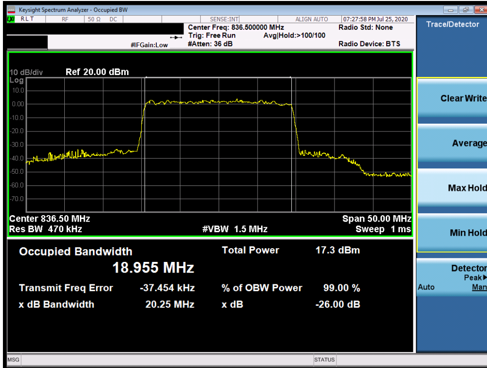
Plot 7-85. Occupied Bandwidth Plot (NR Band n5 - 20.0MHz CP-OFDM 256QAM - Full RB)
