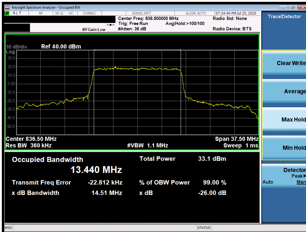
Plot 7-86. Occupied Bandwidth Plot (NR Band n5 - 15.0MHz DFT-s-OFDM BPSK - Full RB)
