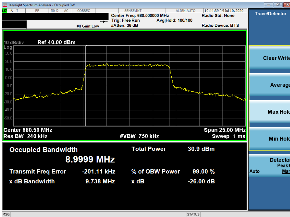
Plot 7-28. Occupied Bandwidth Plot (NR Band n71 - 10MHz CP-OFDM QPSK - Full RB)
