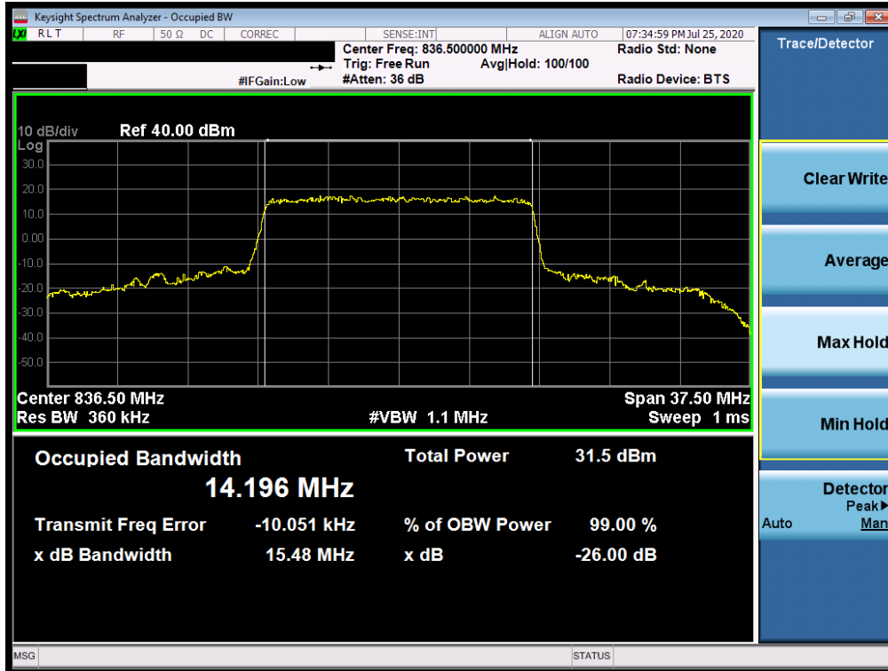
Plot 7-87. Occupied Bandwidth Plot (NR Band n5 - 15.0MHz CP-OFDM QPSK - Full RB)
