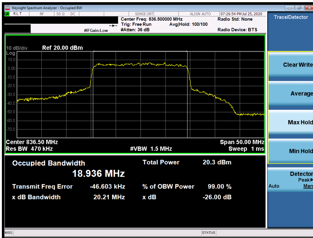
Plot 7-82. Occupied Bandwidth Plot (NR Band n5 - 20.0MHz CP-OFDM QPSK - Full RB)
