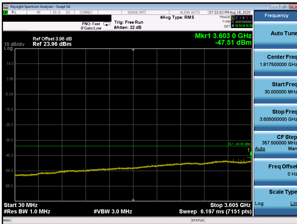
Plot 7-36. Conducted Spurious Plot (LTE Band 48 - 20.0MHz QPSK - RB Size 1, RB Offset 0 - Mid Channel)
