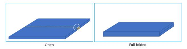
The Powet Sharing mode of the EUT was investigated in two foldable conditions(Open and Full-folded). It was determined that the "Open" condition was the worst-case orientation; therefore all final radiated testing was performed with the EUT in the "Open" condition while generating continuous emissions.
