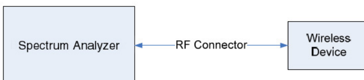
Figure 7-1. Test Instrument & Measurement Setup
