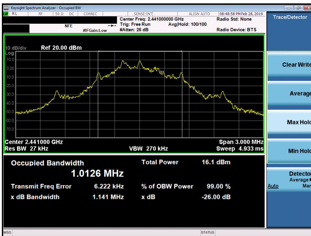
Plot 7-1. Occupied Bandwidth Plot (ANT+ – Ch. 39)
